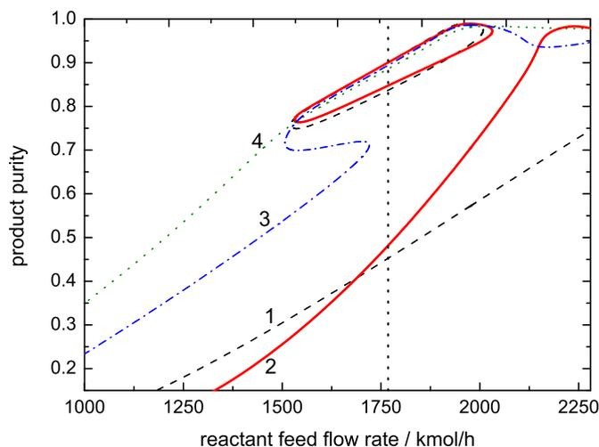
Fig. 7. Product purity vs. butenes flow rate solution diagrams (1 – dashed line – Model 1, 2 – thick solid line – Model 2, 3 – dash – dotted line – Model 3, 4 – dotted line – Model 4).
