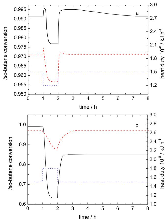
Fig. 6. Isobutene conversion changes predicted by the EQ (solid line) and NEQ (dashed line) models caused by a step decrease (a) and increase (b) of the reboiler heat duty (dotted line) from the operating value and back. Duration of deviations: 1 h.
