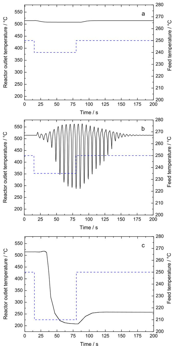
**Fig. 3.** Effect of a reactor response to the failure of inlet feed temperature simulated as step change from the operating value to 240 °C (a), 235 °C (b), and 210 °C (c) (solid lines – reactor outlet temperature, dashed lines – reactor feed temperature).
