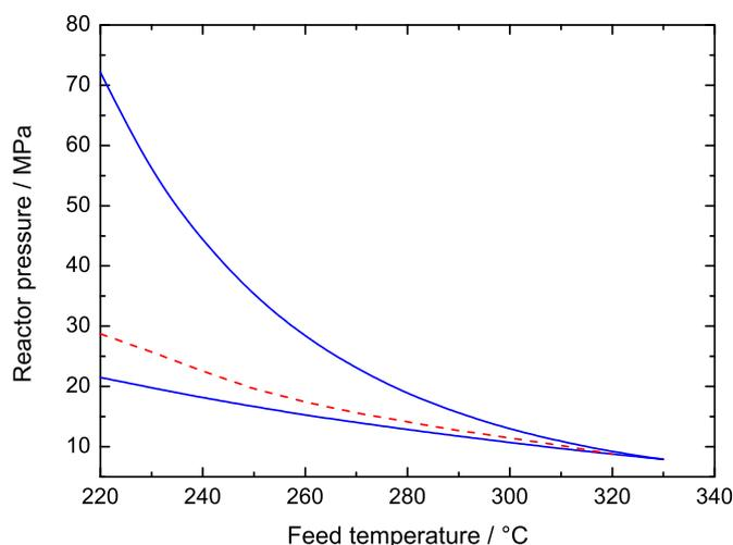
**Fig. 4.** Bifurcation diagram in the parametric plane feed temperature and reactor pressure. The region of multiple steady states is between the solid lines. Dashed line represents the border of the Hopf bifurcation points.
