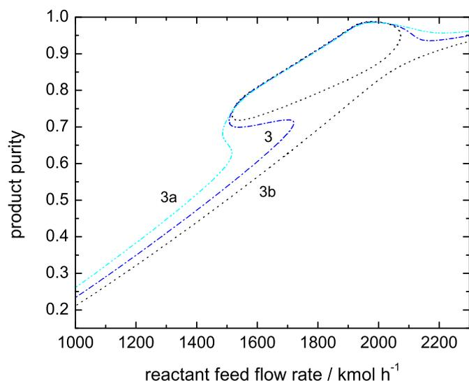
**Fig. 8.** Product purity vs. reactant feed flow rate solution diagrams predicted by Model 3 using different liquid phase diffusion coefficients,  $D^L$ , (3a – dash-dot-dotted line –  $0.8 \times D^L$ , 3 – dash-dotted line –  $1 \times D^L$ , 3b – dotted line –  $1.2 \times D^L$ ).
