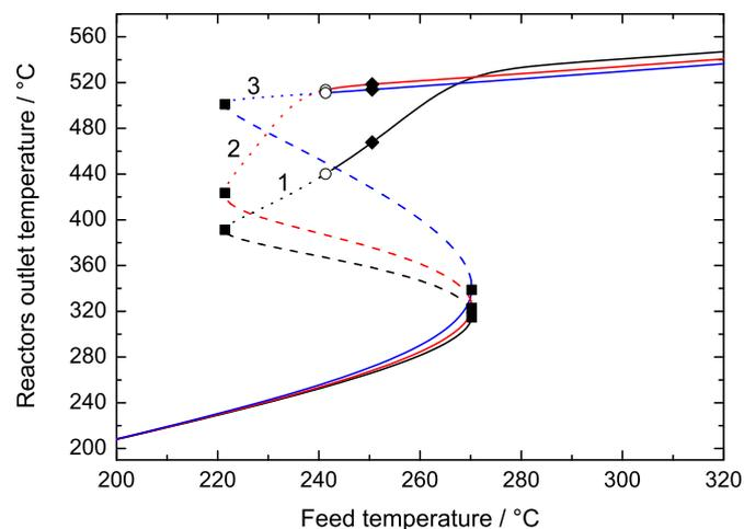
Fig. 2. Solution diagram of reactor segments outlet temperature (1. segment – black line, 2. segment – red line, 3. segment – blue line) as a function of feed temperature (diamonds – normal operating point, empty circles – Hopf bifurcation point, full squares – limit, dashed lines – unstable steady states). (For interpretation of the references to color in this figure legend, the reader is referred to the web version of this article.)
