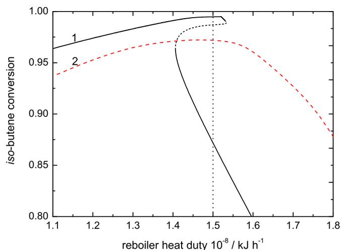
**Fig. 5.** Conversion of isobutene vs. reboiler heat duty solution diagrams predicted by equilibrium (1) and nonequilibrium (2) models.
