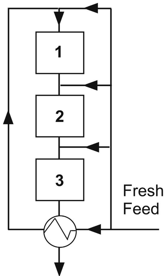
Fig. 1. Schematic description of an ammonia synthesis reactor.
