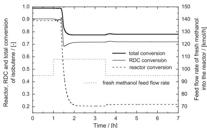
Fig. 4. Deviation: 13.7% higher flow rate of fresh methanol into the fixed bed reactor and back.
