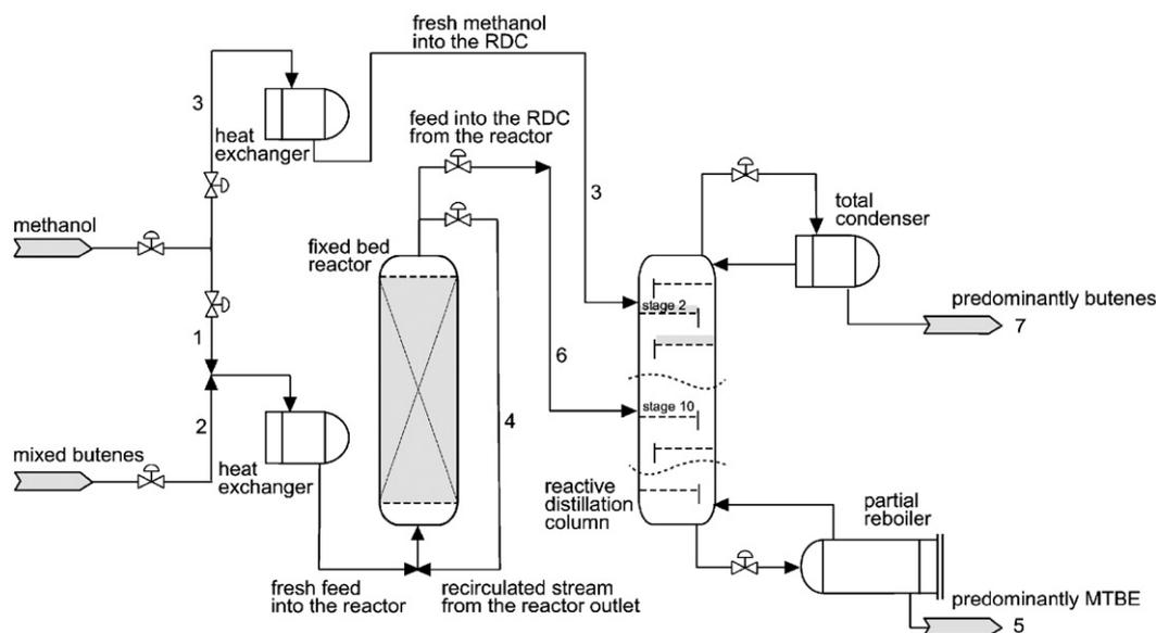
Fig. 1. Schematic flow diagram of the MTBE plant.
