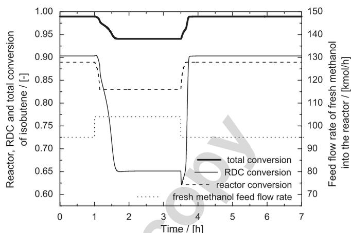
Fig. 3. Deviation: 9.5% higher flow rate of fresh methanol into the fixed bed reactor and back.
