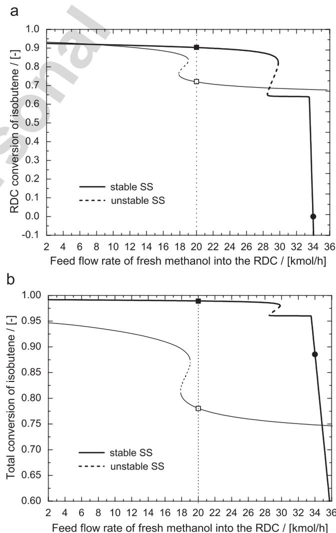
Fig. 6. The solution diagrams of (a) reactive distillation column conversion and (b) total conversion, of IB as a function of fresh methanol feed flow rate into the reactive distillation column (thick curve corresponds with the situation when the fixed bed reactor works at the upper-stable operating point (solid square in Fig. 2a) and the thin curve corresponds with the situation when the fixed bed reactor works at the lower stable operating point (empty square in Fig. 2a)).
