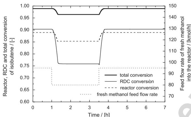
Fig. 5. Deviation: 15.8% lower flow rate of fresh methanol into the fixed bed reactor and back.
