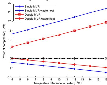
Fig.4 Standard coal needed by single, double-stage MVR system with the temperature difference in the heater
