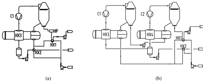
Fig. 1 Single-stage and Double-stage MVR process with self-heat recuperation technology
