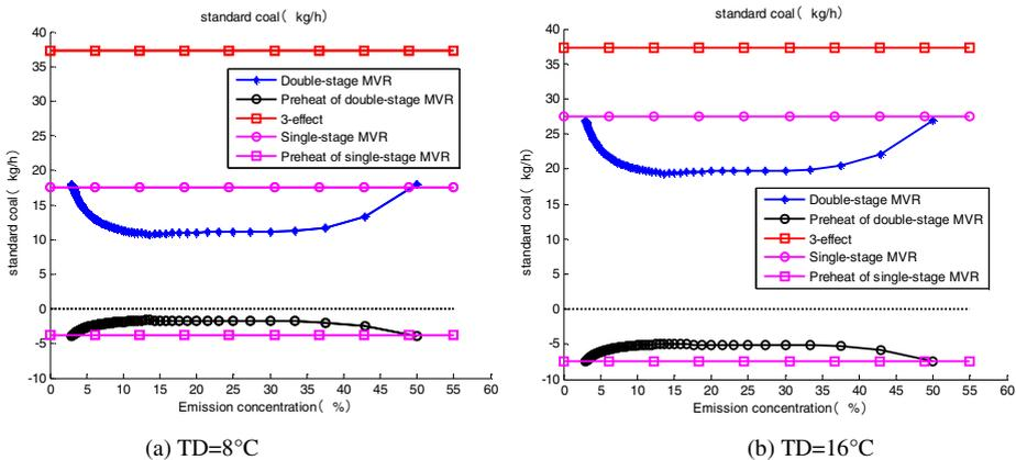
Fig. 3 Standard coal needed at different temperature difference in the heater for three systems
