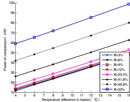
Fig. 2 Power of compressor for 1000kg/h vapor with temperature difference in heater
