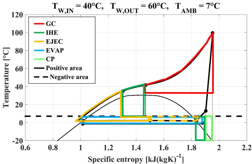
Fig. 5. Exergy losses  $\pi$  in the  $T$ - $s$  diagram for transcritical  $CO_2$  multi-ejector cycle.
