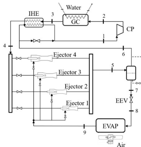
Fig. 1. Layout of multi ejector expansion CO<sub>2</sub> vapour compression system test setup.
