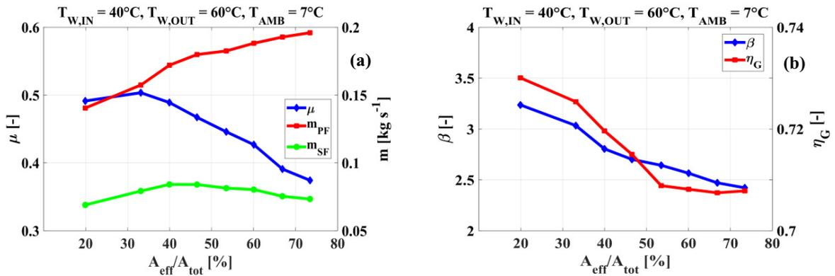
Fig. 3. Performance variations as a function of the overall ejectors cross section. 3.a) entrainment ratio (left) and mass flow rates (right); 3.b) pressure ratio (left) and compressor global efficiency (right).
