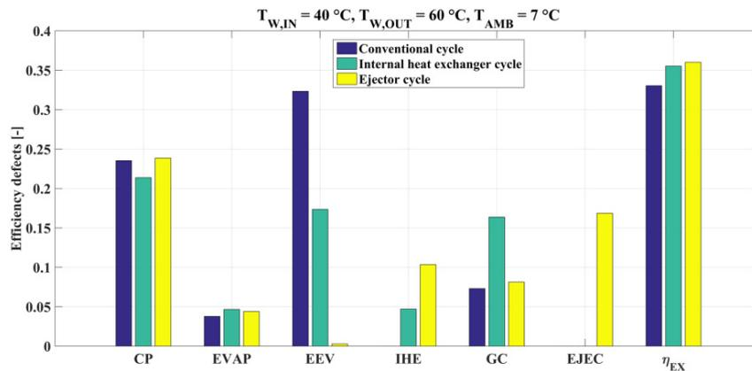
Fig. 7. Exergy losses comparison between ejector cycle, expansion valve cycle and internal heat exchanger, in the maximum ejector efficiency configuration.
