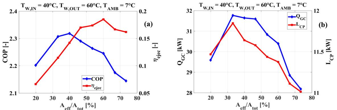
Fig. 4. Performance variation as a function of the overall ejectors cross section. 4.a) COP (left) and ejector efficiency (right); 4.b) heating capacity (left) and compression work (right).
