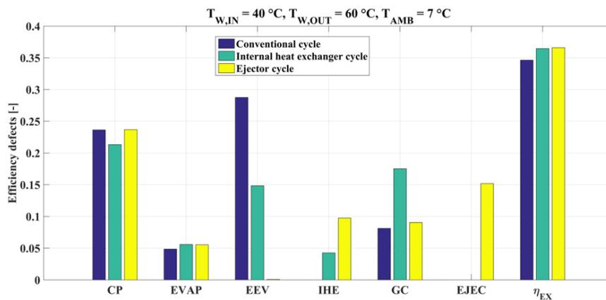
Fig. 6. Exergy losses comparison between ejector cycle, expansion valve cycle and internal heat exchanger, in the maximum COP configuration.
