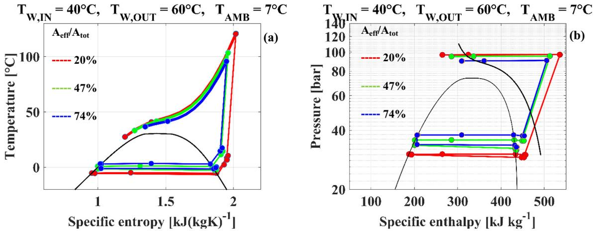
Fig. 2. (a) T-s diagram and (b) p-h diagram, variation of the thermodynamic cycle varying the overall ejectors cross section for fixed boundary conditions, represented on the top of the figure.
