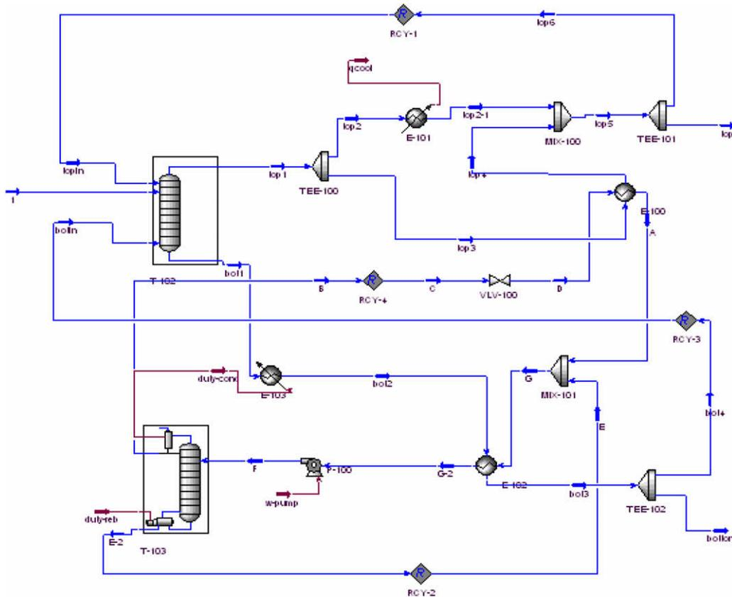
Fig. 4. HYSYS process flow diagram for the absorption heat pump.
