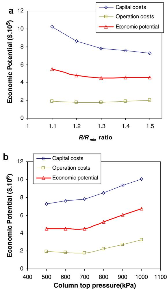
Fig. 7. (a) Variation of economic potential with column reflux ratio for the bottom flashing heat pump. (b) Variation of economic potential with column pressure for the bottom flashing heat pump.
