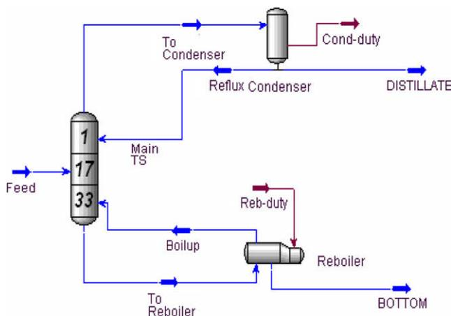
Fig. 1. HYSYS process flow diagram for the conventional column.
