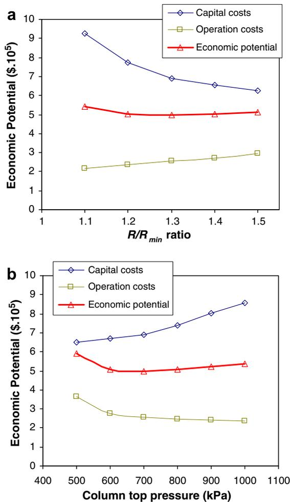
**Fig. 5.** (a) Variation of economic potential with column reflux ratio for the conventional distillation. (b) Variation of economic potential with column pressure for the conventional distillation.
