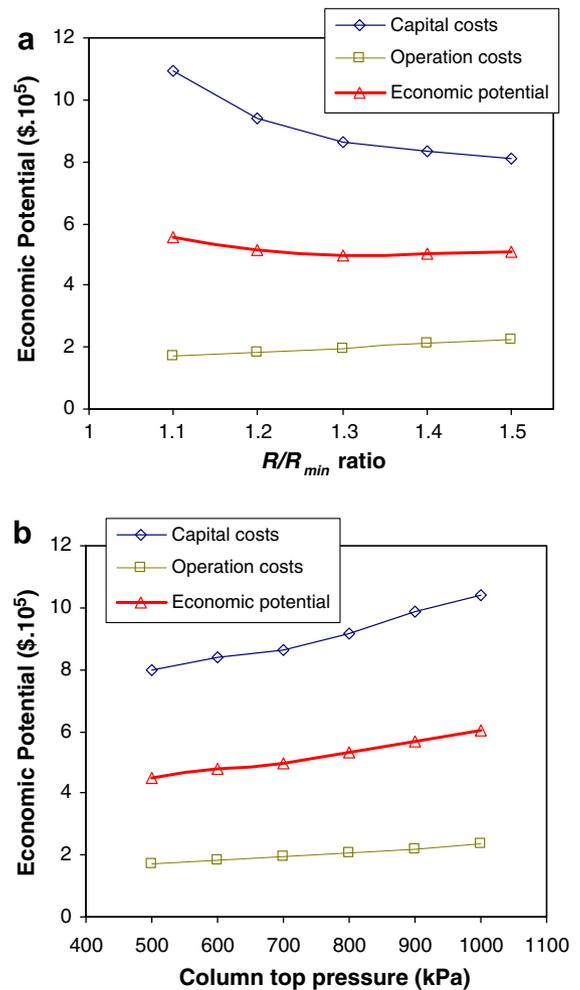
**Fig. 6.** (a) Variation of economic potential with column reflux ratio for the vapour recompression heat pump. (b) Variation of economic potential with column pressure for the vapour recompression heat pump.
