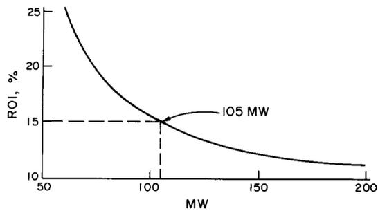
Fig. 2. Projected return on investment vs megawatt size 1985 pulverized coal-fired industrial power plant.
