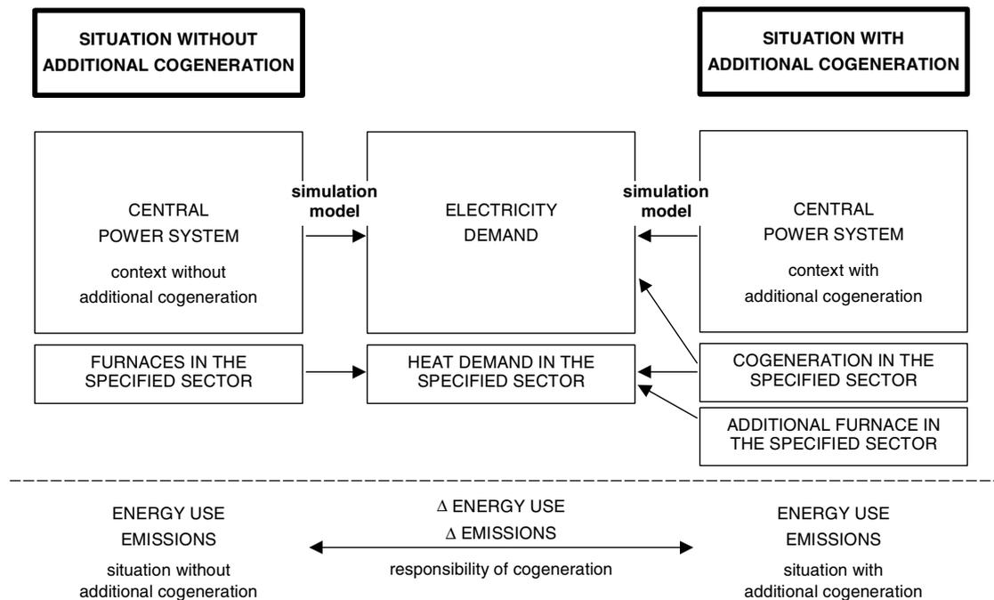
Fig. 1. Method for the evaluation of cogeneration. The scenario on the left hand side is the base case without additional cogeneration. The scenario on the right hand side is the alternative scenario with additional cogeneration. In both scenarios, the same energy—heat and electricity—is delivered (see [1,2] for more details).
