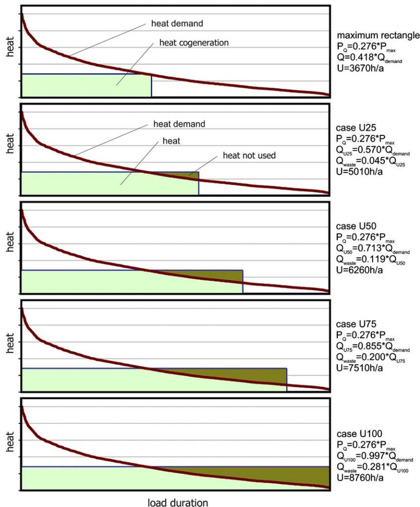
Fig. 7. Partial-heat-usage sizing of cogeneration. The annual use in the four alternative cases gradually increased from 3670 h/a in the “maximum-rectangle” case to 5010 h/a, 6260 h/a, 7510 h/a and finally the full 8760 h/a for case U25, case U50, case U75 and case U100, respectively.
