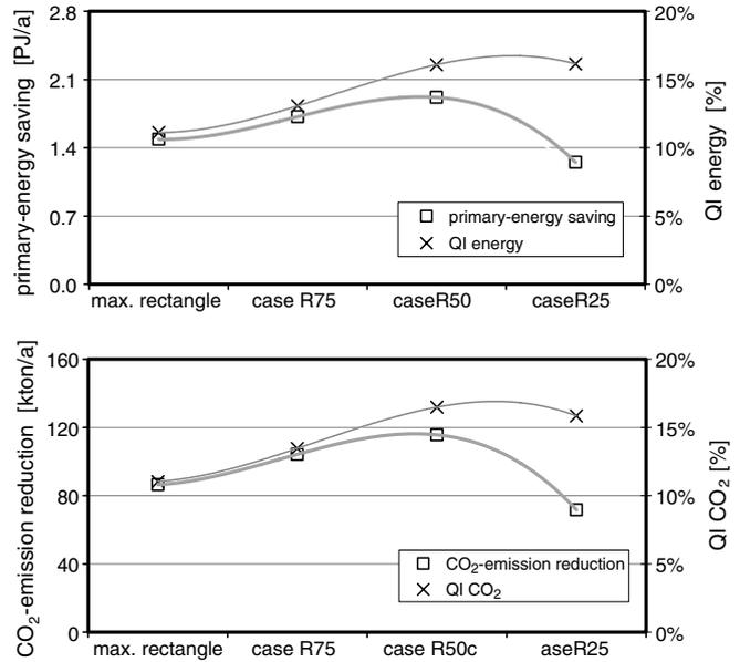
Fig. 6. Results of the scenarios with reduced-sale sizing of cogeneration compared to the results obtained by using the “maximum-rectangle” rule for cogeneration in the service sector.
