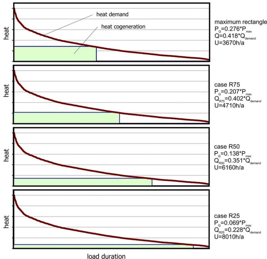
Fig. 5. Reduced-scale sizing of cogeneration. The thermal power of the three alternatives is 75%, 50% and 25% of the rated thermal power in the “maximum-rectangle” case in the top figure for case R75, case R50 and case R25, respectively.
