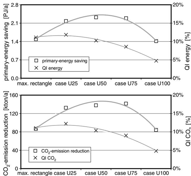
Fig. 8. Results of the scenarios with partial-heat-usage sizing of cogeneration compared to the results obtained by using the “maximum-rectangle” rule for cogeneration in the service sector.
