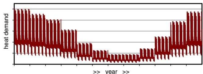
Fig. 2. Typical chronological heat-demand profile in the service sector. The horizontal axis covers a full year, the ordinate axis uses arbitrary normalised units.
