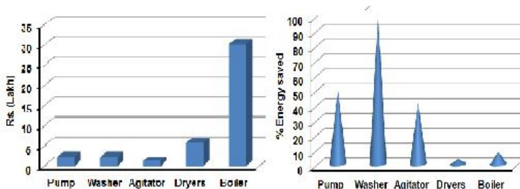
**Fig. 1:** Cost and Energy saving for the audited sections.
