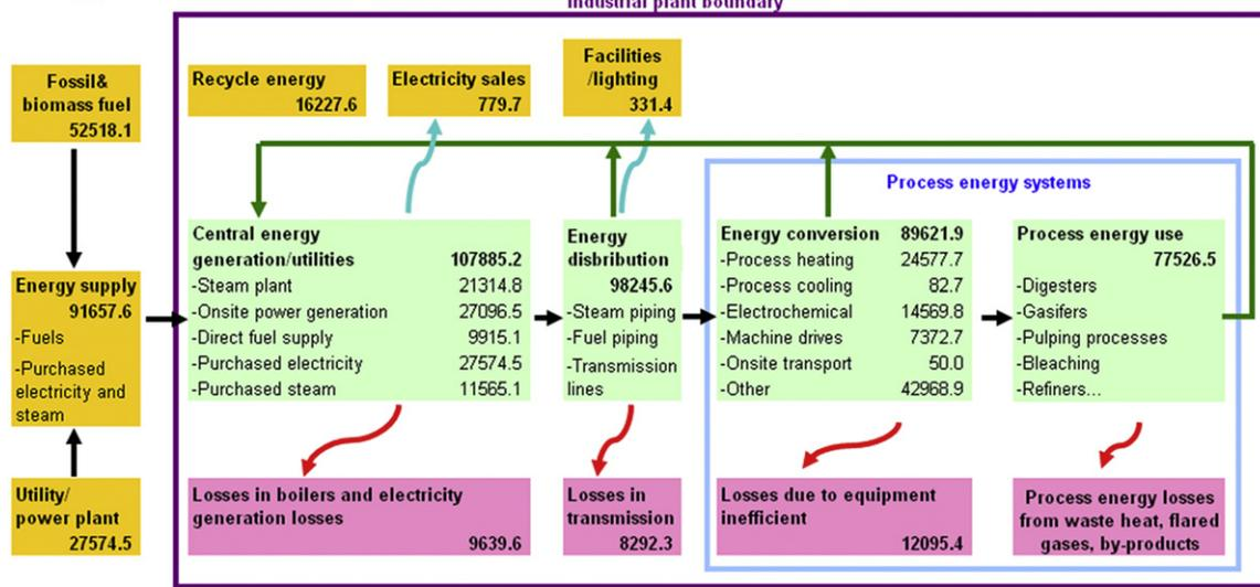
Fig. 2. Energy flow profile of Taiwanese pulp and paper industry (Energy unit: KLOE/M).
