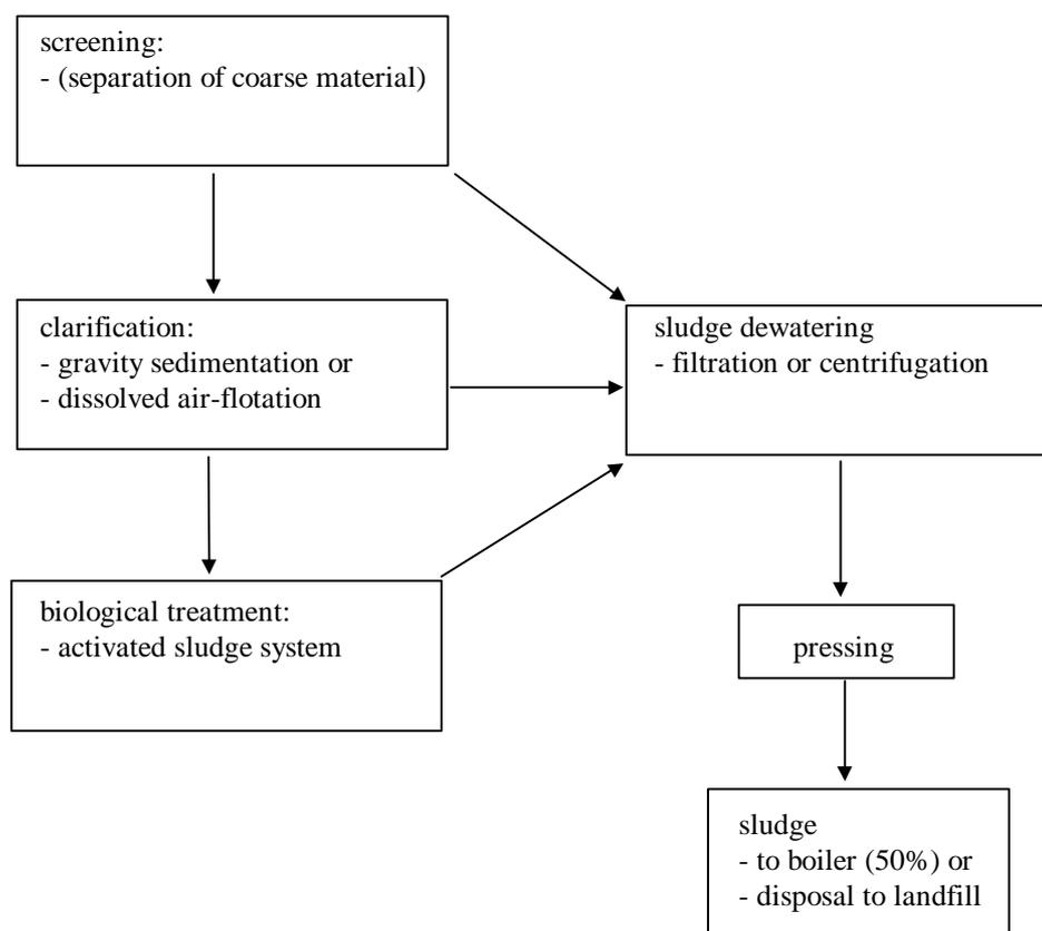
Activated sludge treatment, which represents 90% of the waste water treatment in Finland, produces 10-15 kg of sludge/ADt (ADt = air dry tonne). In 90% of the mills, sludge is incinerated in boilers. The real energy consumption of effluent treatment is 60-80 kWh/ADt including electricity and heat. The energy consumption for the biological treatment is as follows
