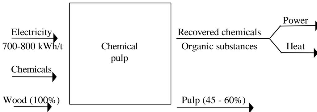
The recovery of chemicals is associated with energy production from combustion of the spent liquor in the soda boiler. This means that a modern chemical pulp plant produces steam and electricity (in back pressure turbines) to the extent needed for the entire plant. In many cases the pulp plant is integrated with a paper production plant and the excess steam from the pulp production is used for drying of paper.
