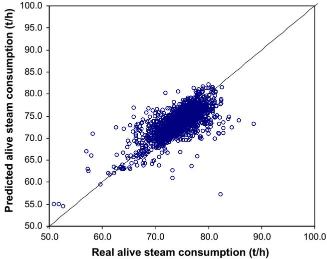
Fig. 4. Comparison between measured and simulated values for the steam consumption in the evaporation system.
