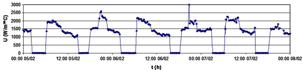
Fig. 6. Simulation of the overall heat transfer coefficient during 4 days of traditional cycle time operation in the evaporation A body (8 h of continuous operation and 4 h of washing).
