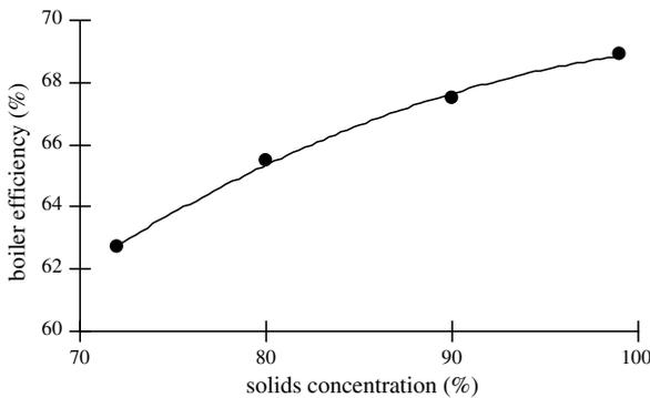
Fig. 8. Simulated value of the boiler thermal efficiency as a function of the solids content in the black liquor feeding the recovery boiler.
