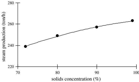
Fig. 7. Simulated value of the superheated steam production rate as a function of the solids concentration in the black liquor feeding the recovery boiler.
