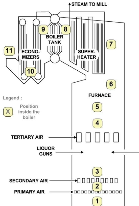
Fig. 10b. Positions inside the boiler at which the operation temperature has been simulated by WinGEMS (shown in Fig. 10a).
