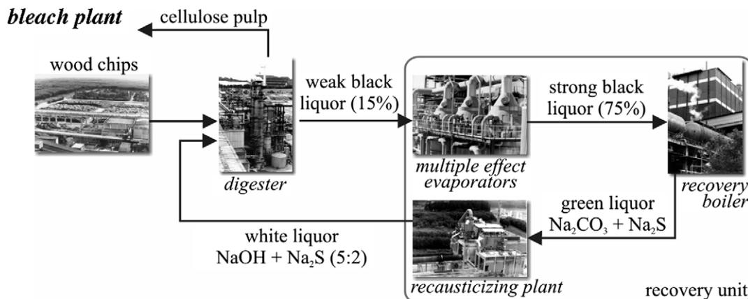
**Fig. 1.** Schematic representation of the pulp mill plant.
