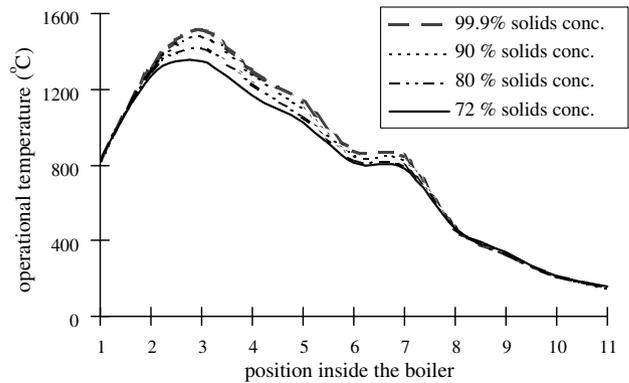
Fig. 10a. Simulated profile of the recovery boiler operational temperature as a function of the solids content in the liquor feed (positions identified in Fig. 10b).
