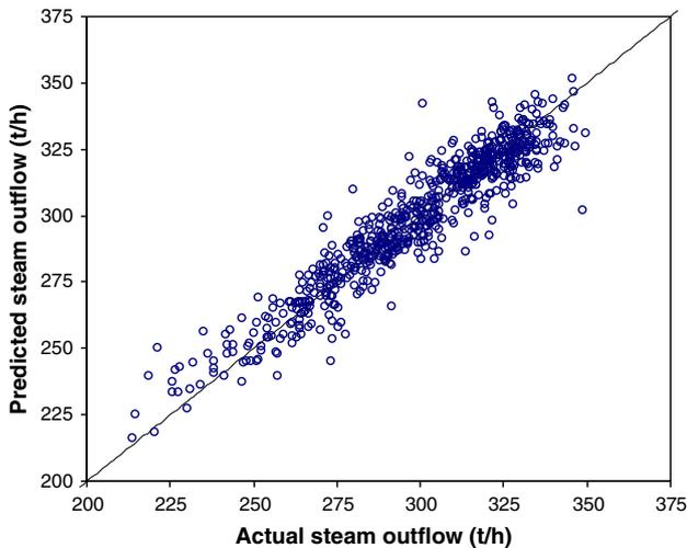
Fig. 5. Comparison between measured and simulated values of the outflow of steam generated in the boiler recovery.
