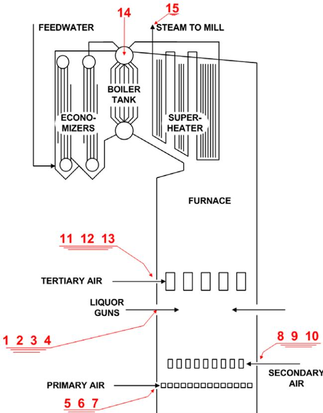
Fig. 3. Sampling points in the recovery boiler for variables shown in Table 3 (boiler diagram after Adams et al. [5]).
