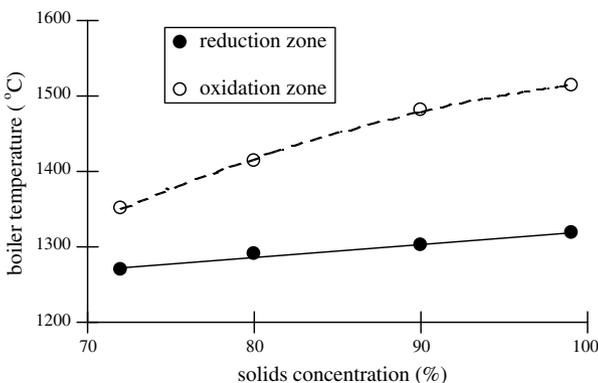
Fig. 9. Simulated value of the operational boiler temperature in the oxidation and reduction zones as a function of the solids content in the liquor feeding the recovery boiler.
