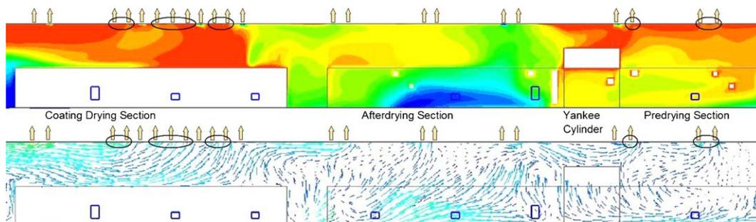
Fig. 7. Temperature and velocity field along the hall and the positions of optimal heat exchangers' intake connections.
