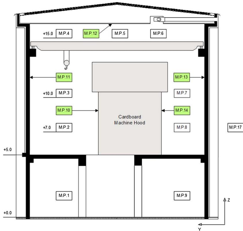
Fig. 1. Locations of the measuring points across one characteristic cross-section of the cardboard machine hall.
