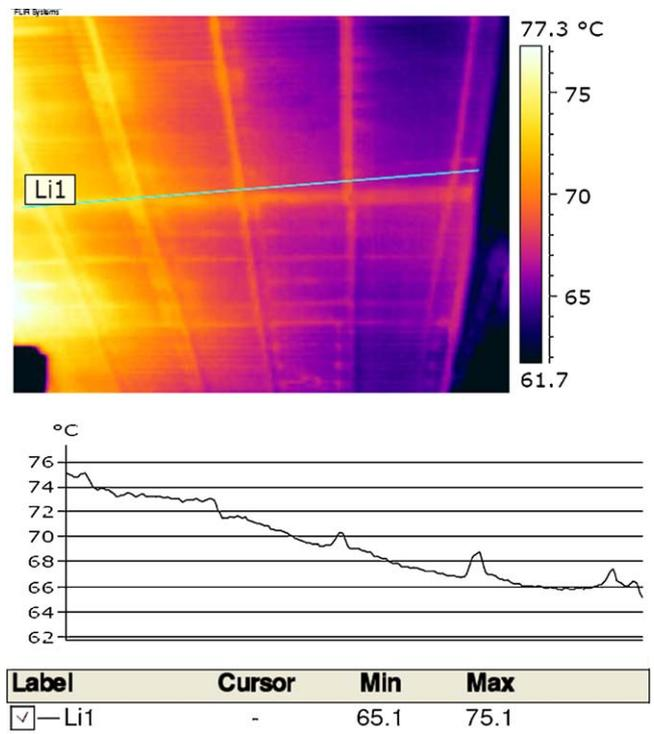
Fig. 3. Ceiling temperature (M.P.12) in coating drying section; temperature increases from northern to southern side of the hall.
