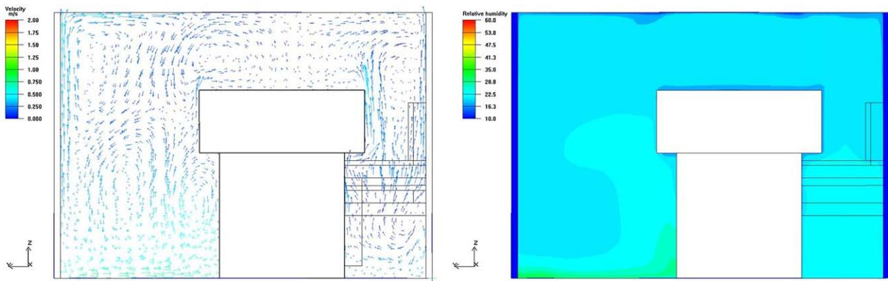
Fig. 6. Simulated velocity distribution and relative humidity in smoothing cylinder section.
