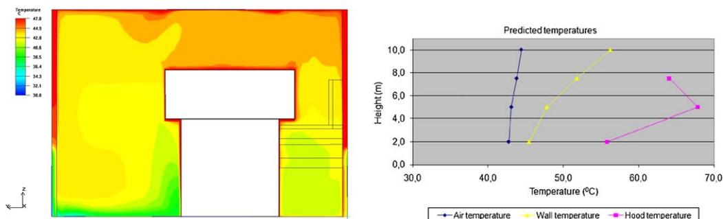
Fig. 5. Simulated temperature distribution in smoothing cylinder section.
