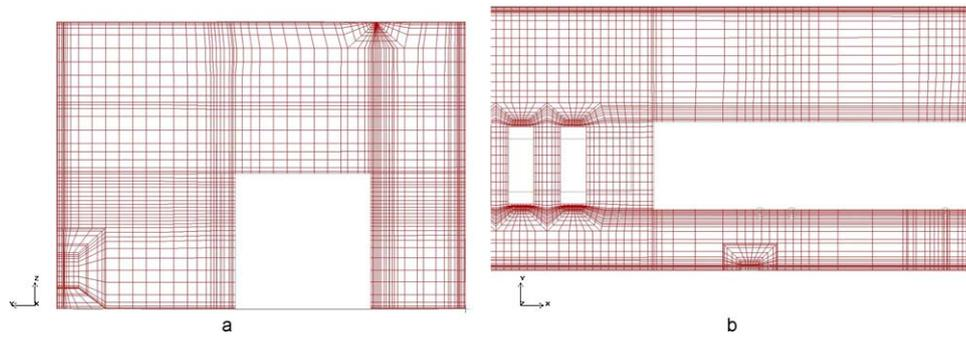
Fig. 4. Mesh configuration in former section; (a) vertical; (b) horizontal.
