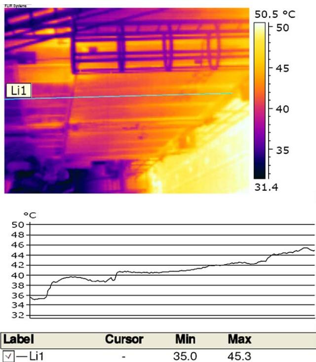
Fig. 2. Temperature of cardboard machine hood (M.P.10) in pre-drying section; temperature increases with hood height.
