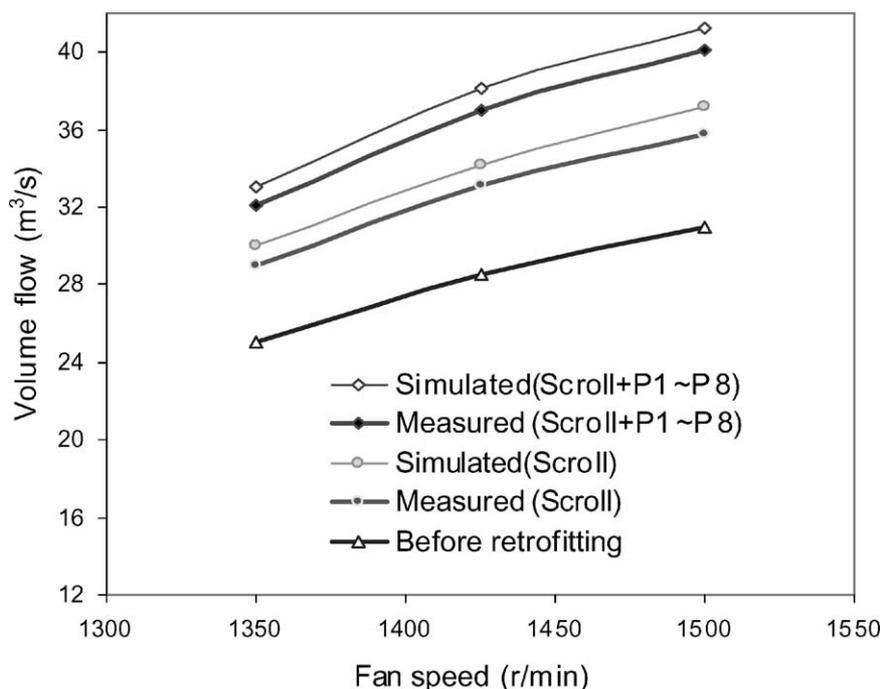
Fig. 11. Comparison between simulated and measured total air volume flow rate before and after installing the fan scroll and splitter vanes in building #2.
