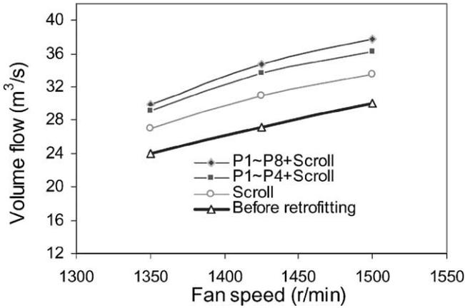
Fig. 9. Simulated total volume flow rate vs. fan speed before and after adding the fan scroll and splitter vanes.
