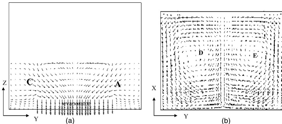
Fig. 3. The simulated velocity vector in the evaporator chamber. (a) In the  $z$ - $x$  plane-elevation; (b) in the  $x$ - $y$  plane-plan form.
