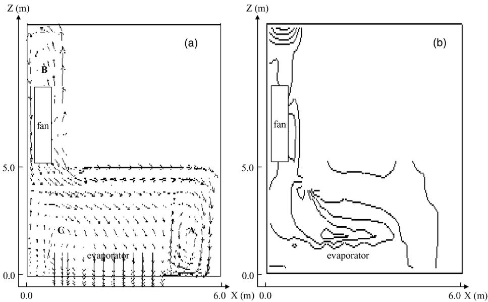
Fig. 2. Simulated velocity of airflow (a) and airflow field (b) at the  $z$ - $x$  plane ( $y = 3.2$  m) in the evaporator chamber before retrofitting.
