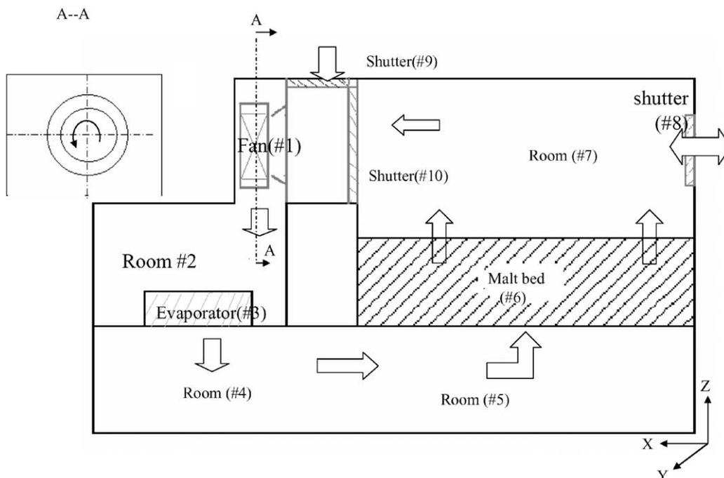
Fig. 1. A (vertical) cross-section sketch of the malt building, top right is a cross-section sketch of the fan.
