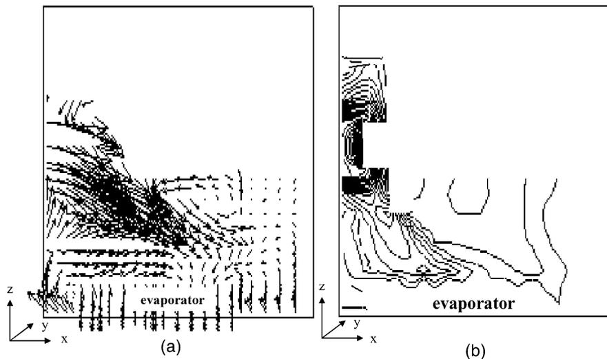
Fig. 6. The velocity vector of the airflow (a) and the airflow field (b) in the evaporator room (at  $z = 0.8$  m) after fan retrofitting.
