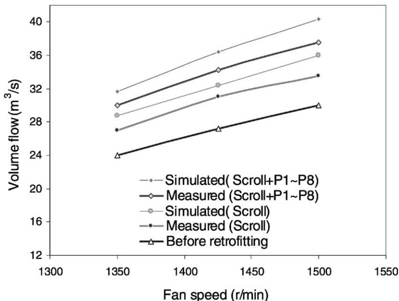
Fig. 10. Comparison between simulated and measured total air volume flow rate before and after installing the fan scroll and splitter vanes in building #1.
