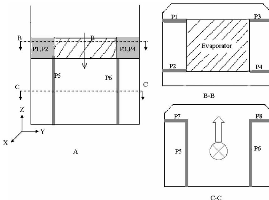
Fig. 8. Illustration of designed splitter vanes installed in the evaporator room and the room below the evaporator.
