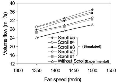
Fig. 5. The simulated system volume flow rate vs. fan speed when adding different scrolls.
