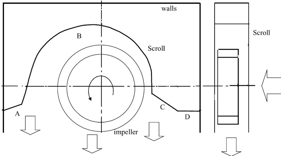
Fig. 4. A cross-section sketch of the fan chamber with the scroll designed.
