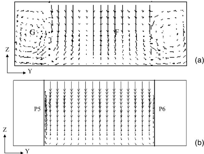
Fig. 7. Simulated velocity in the room below the vaporator in the  $z$ - $y$  plane (elevation) before (a) and after (b) installing plates P5 and P6.
