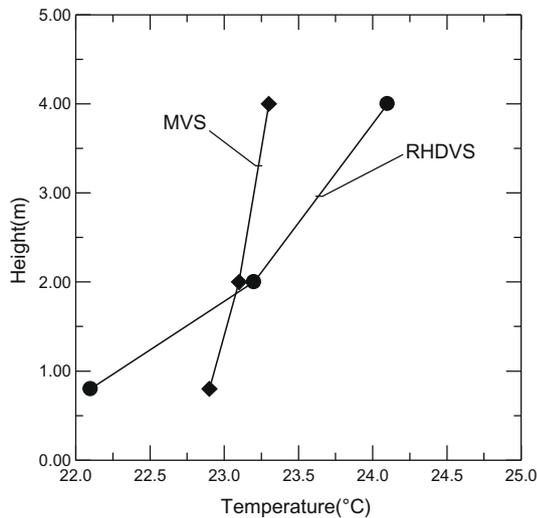
Fig. 10. Vertical temperature gradient (RHDVS and MVS comparison).
