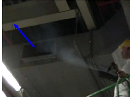
**Fig. 6.** Smoke injection at duct level.
