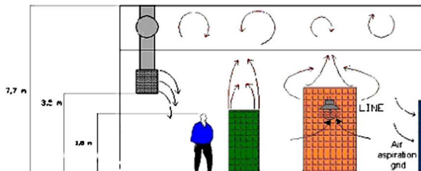
Fig. 2. Scheme of the hybrid displacement ventilation system.
