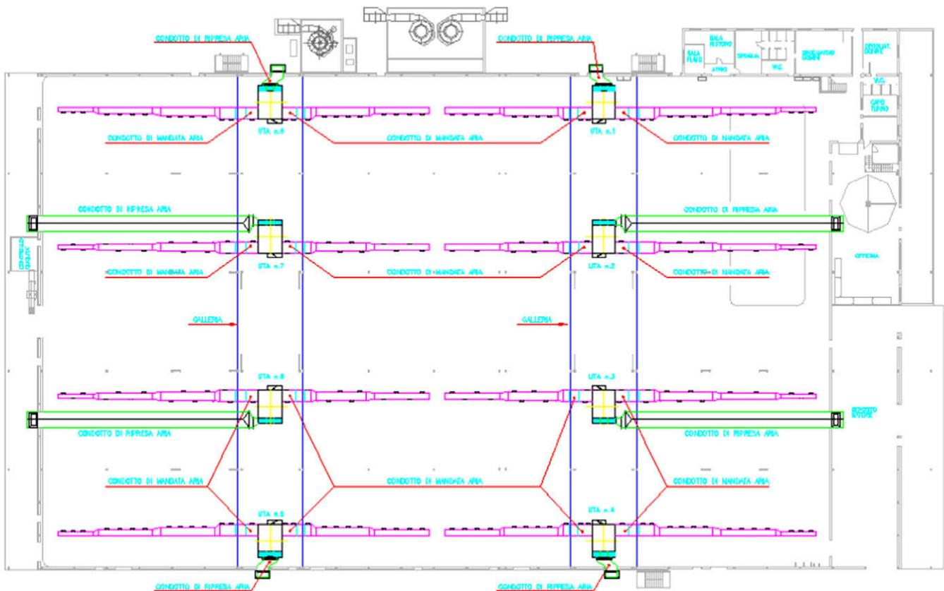
Fig. 5. Layout of air distribution channels.
