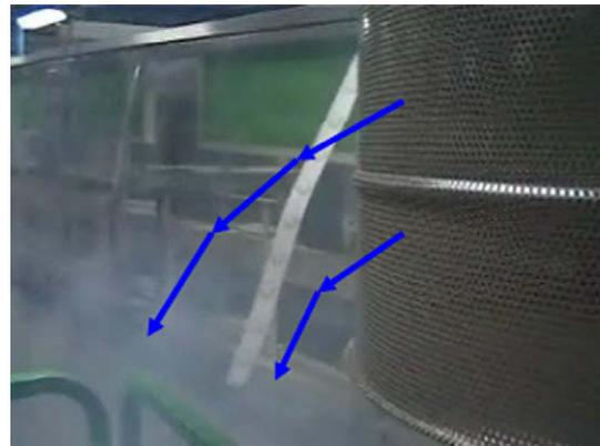
Fig. 14. Smoke flow visualization experiments with the text diffuser.
