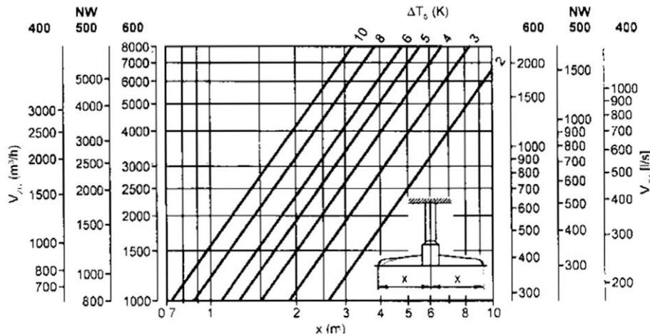
Fig. 3. Typical flow characteristics of diffuser with horizontal air ejection (NW = diffuser diameter in mm).
