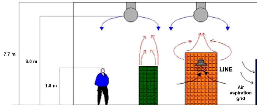
Fig. 1. Scheme of mixing ventilation system.
