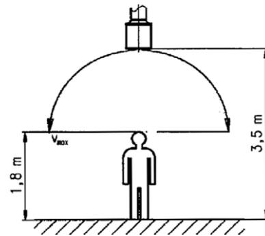
Fig. 4. Typical flow pattern of a ceiling mounted diffuser.
