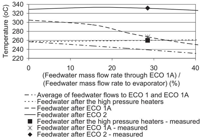
Fig. 8. Calculated and measured feedwater temperatures at various locations.
