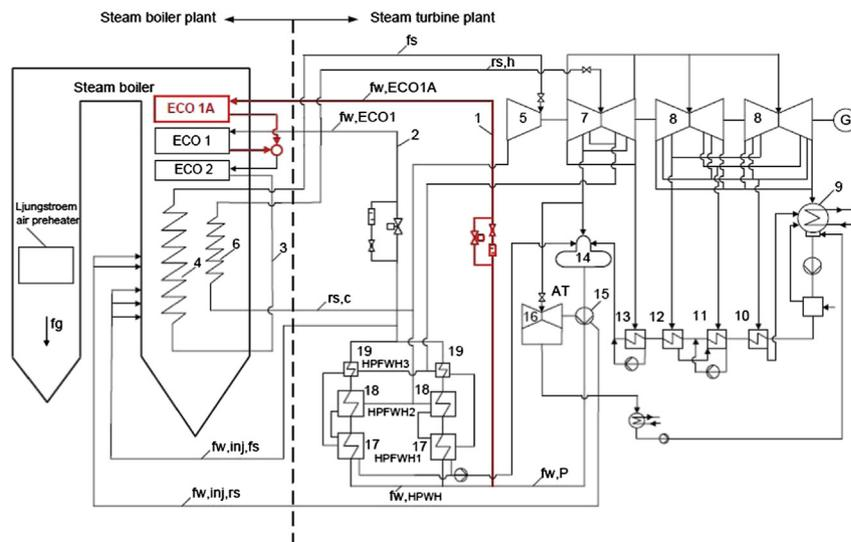
Fig. 3. Additional economizer ECO 1A installation at Unit B1 of the Thermal Power Plant "Nikola Tesla B".
