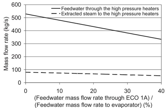
Fig. 7. Feedwater mass flow rate through the high pressure heaters and the corresponding mass rate of extracted steam condensation.
