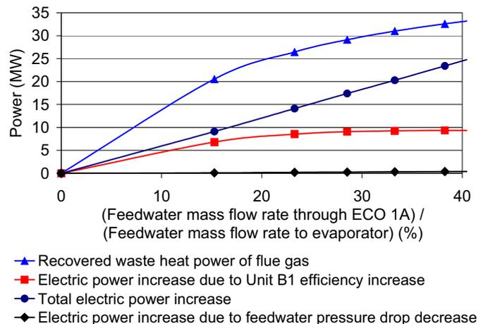
Fig. 10. Recovered waste heat power and corresponding electric power upgrade by the installation of the additional economizer.
