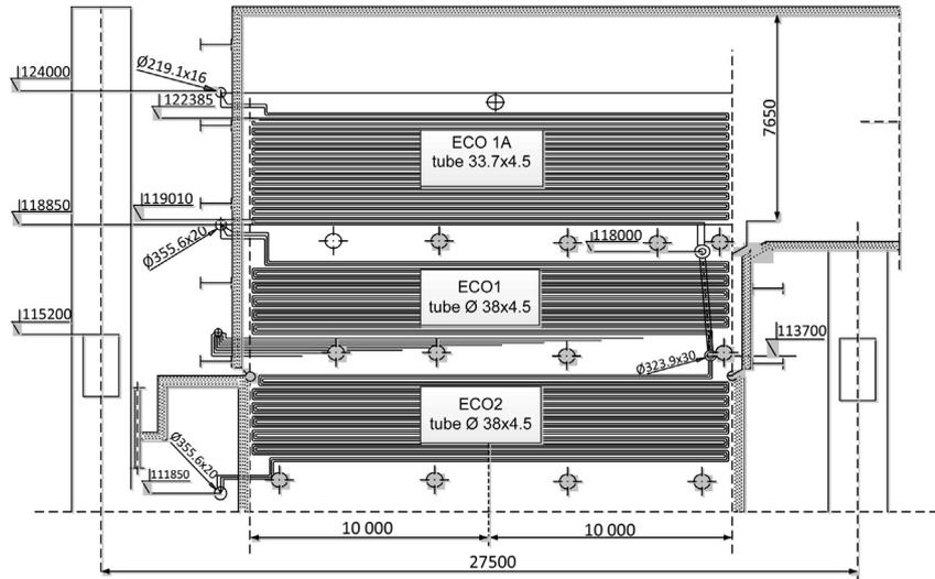
Fig. 4. Layout of the additional economizer ECO 1A.
