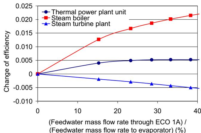
Fig. 11. Efficiency upgrade by the installation of the additional economizer.
