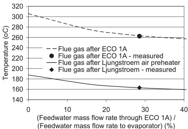
Fig. 9. Calculated and measured flue gas temperatures after additional economizer and the Ljungstrom air preheater.
