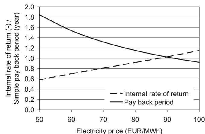
Fig. 12. Internal rate of return and simple pay back period dependence on the electricity price.
