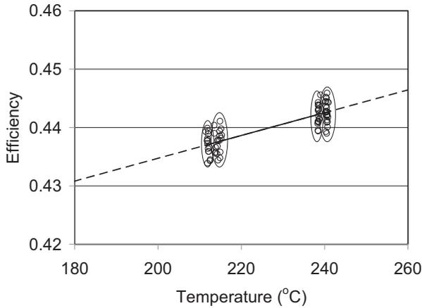
Fig. 6. Steam turbine plant efficiency in dependence of the mean feedwater temperature (mean temperatures calculated from the mean enthalpies (Eq. (9)) of the feedwater flows into the originally built economizer ECO 1 and the additional economizer ECO 1A).
