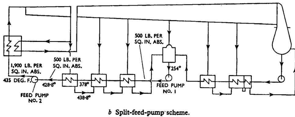
Fig. 3. Feed Heating Systems for Reheat Cycle
