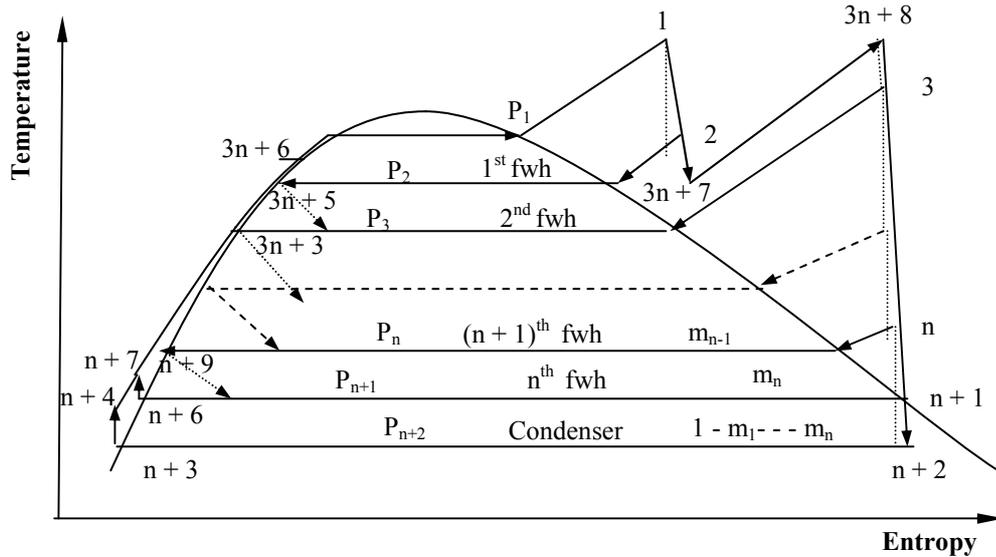
Figure 2. Temperature-entropy diagram of Rankine cycle with 'n' fwhs and a reheater
