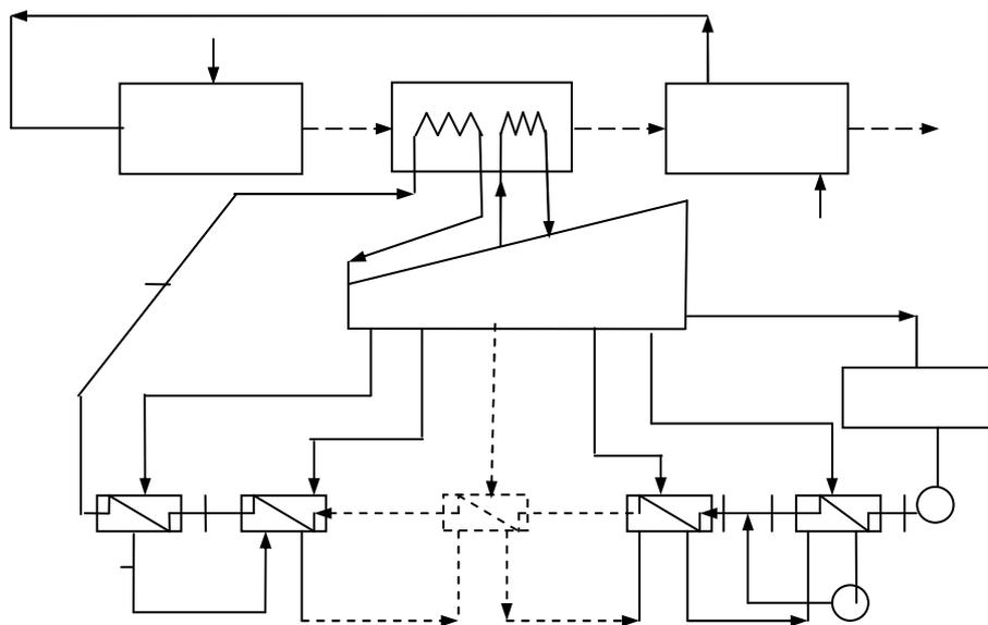
*Figure 1. Schematic flow diagram of steam cycle with 'n' fwhs and a reheater*
