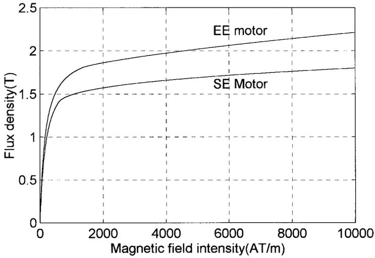
Fig. 1. Magnetizing characteristics of EE and SE motors.
