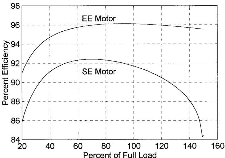
Fig. 6. Comparison of efficiency versus load level characteristics of EE and SE motors.
