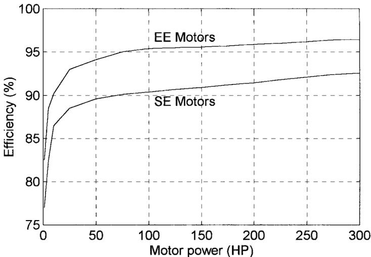
Fig. 3. Comparison of the efficiency of EE and SE motors.
