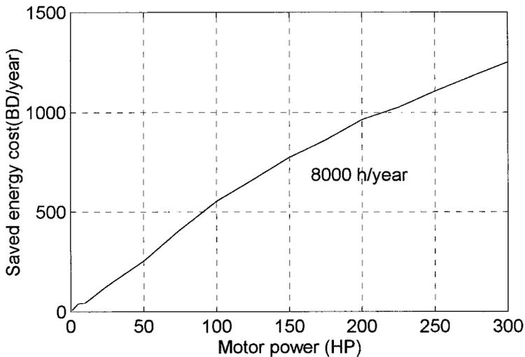
Fig. 5. Variation of the saved energy cost with motor size.
