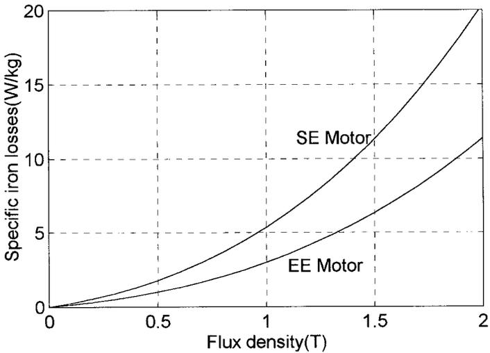
Fig. 2. Specific iron losses of EE and SE motors.
