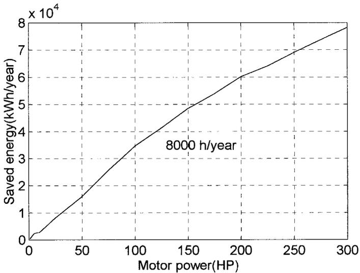
Fig. 4. Variation of the saved energy per-year with the motor size.
