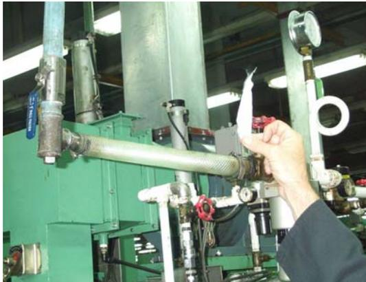
a. leaks at rubber hose connection
