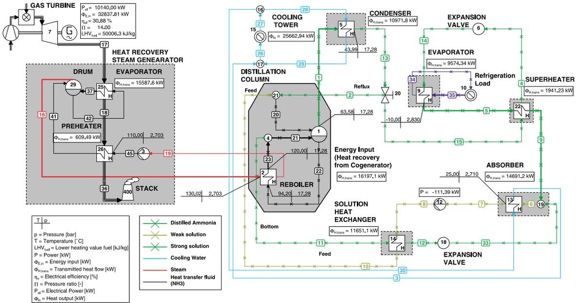
Fig. 5. Process flow diagram of the trigeneration system composed by a gas turbine, an HRSG and an ammonia water absorption plant. The highlighted operating parameters are the result of the thermodynamic optimization.
