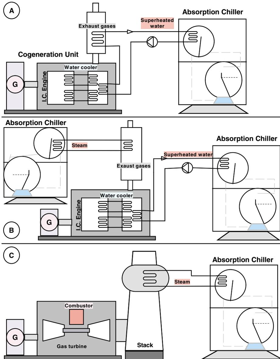
Fig. 1. Possible configurations of a trigeneration system based on an AAR plant.
