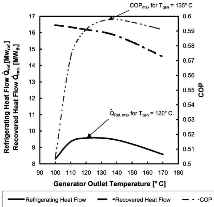
Fig. 6. Refrigerating heat flow and COP of the AAR cycle together with the recovered heat flow from the gas turbine as a function of the generating temperature, which is also bound to the HRSG pressure.
