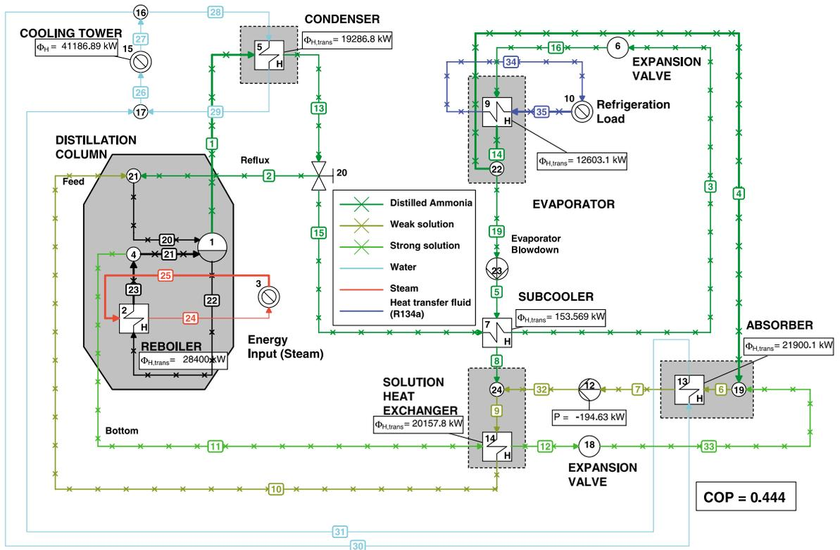
Fig. 2. Process flow diagram of an ammonia water refrigeration cycle: evaporator blowdown is dumped to the absorber section. Displayed results are calculated with *Cycle-Tempo* [8] and are used for validation against calculations published in [12]. Design data and configuration in [12] are taken from [13] and concern an ammonia manufacturing plant.
