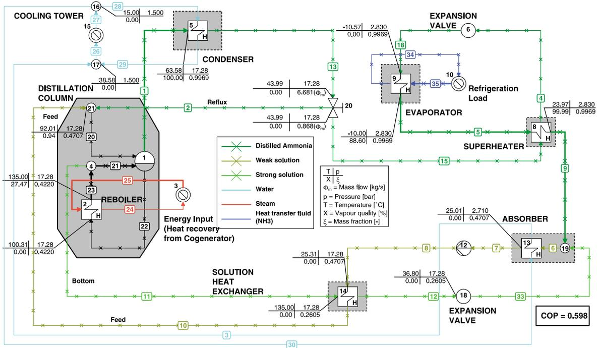
Fig. 3. Process flow diagram of the single stage AAR cycle considered for the coupling with cogenerators. The configuration includes refrigerant pre-cooling made using spent vapor from the evaporator.
