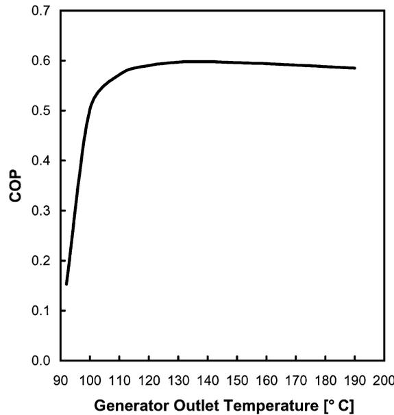
Fig. 4. Effect of the generator (reboiler) temperature on COP for the single stage AAR cycle of Fig. 3. Operating parameters are listed in Table 4.
