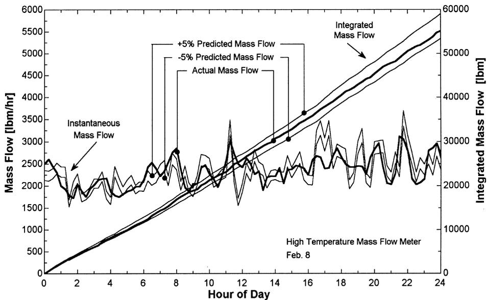
Fig. 5. Comparison of calculated and measured refrigerant mass flows in the high temperature circuit.
