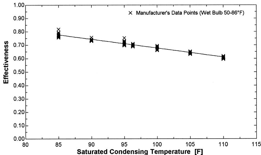
Fig. 4. Evaporative condenser effectiveness as a function of condensing temperature (the effectiveness can be fit to a linear function of condensing temperature with  $R^2 = 95.9\%$ ).
