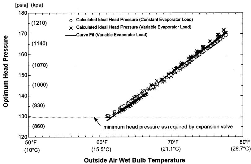
Fig. 11. Optimum head pressure setpoints as a function of wet-bulb temperature.
