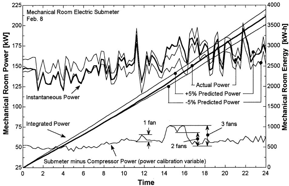
Fig. 6. Comparison of calculated and measured mechanical room power.
