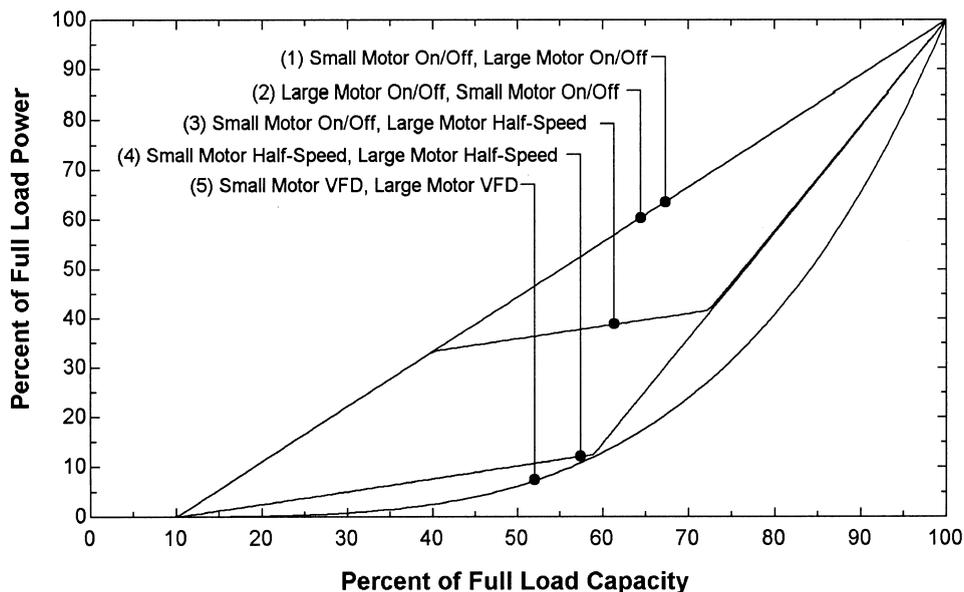
Fig. 8. Part-load evaporative condenser operation.
