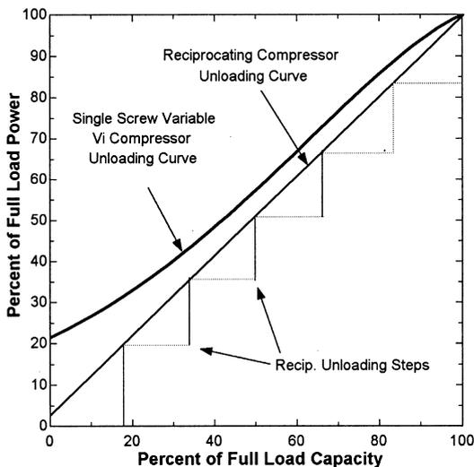
Fig. 2. Part-load performance of the screw and reciprocating compressor.
