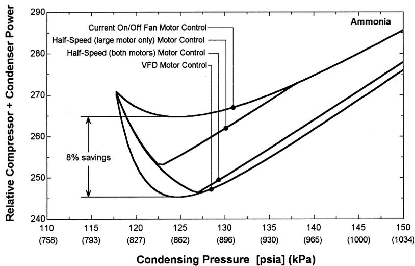
Fig. 9. Evaporative condenser fan motor control strategies for an average day in May.
