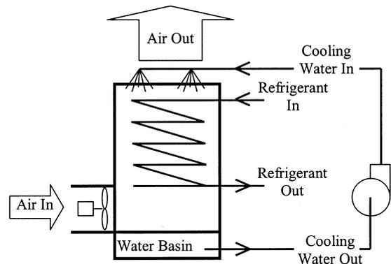
Fig. 3. Schematic representation of the evaporative condenser.
