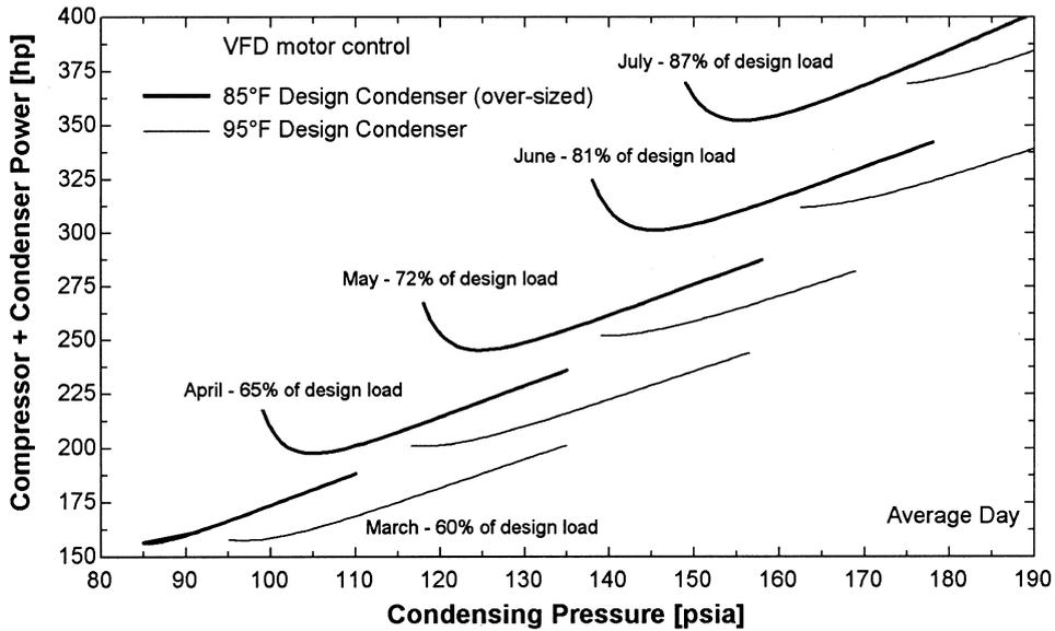
Fig. 10. Optimum condensing pressure for varying loads and outside air conditions.
