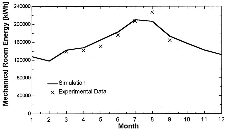
Fig. 7. Comparison of measured and simulated engine room monthly energy use.
