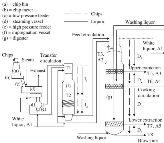
Fig. 1. Continuous cooking application with impregnation vessel and digester.
