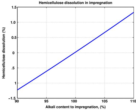
Fig. 8. Hemicellulose dissolution in impregnation in different alkali dosages.
