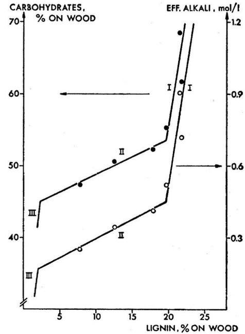
Fig. 2. Carbohydrate yield (% on dry wood) and effective alkali concentration in cooking liquor as a function of lignin content (% on dry wood). Olm and Tistad [1979]
