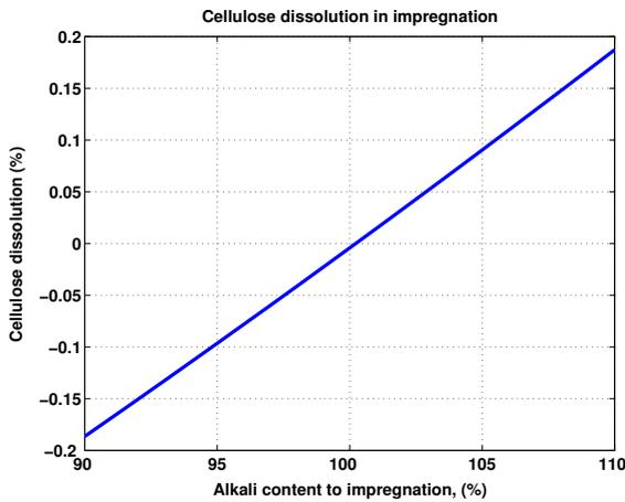
Fig. 9. Cellulose dissolution in impregnation in different alkali dosages.
