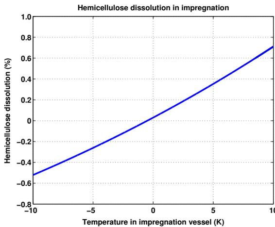
Fig. 10. Hemicellulose dissolution in impregnation in different temperatures.
