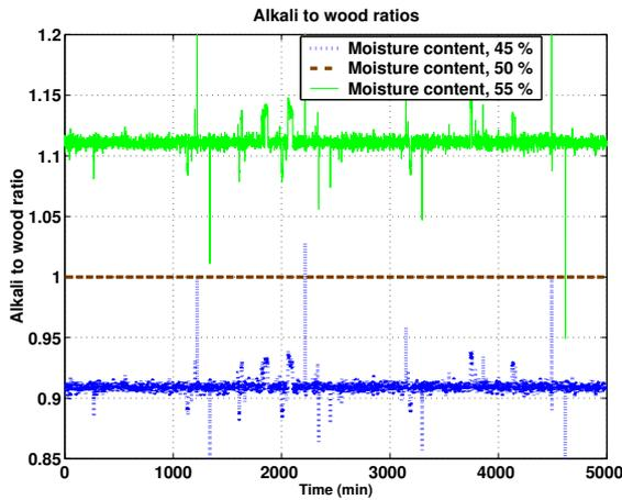
Fig. 3. Alkali to wood ratio, if the moisture content is changed from 45% to 55%.
