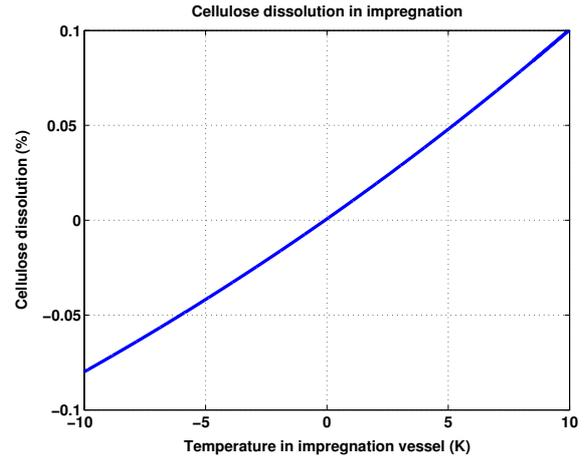
Fig. 11. Cellulose dissolution in impregnation in different temperatures.
