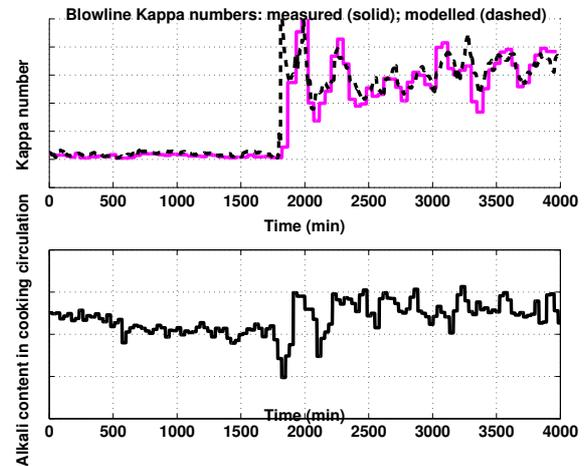
Fig. 12. Blow line Kappa number vs alkali content in cooking circulation.
