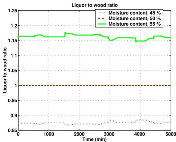
Fig. 4. Liquor to wood ratio, if the moisture content is changed from 45% to 55%.
