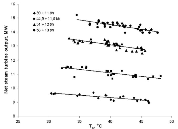
Fig. 6. Steam turbine output minus combined cycle's parasitic load as a function of steam condensing temperature for various HP + MP steam generation rates.
