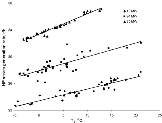
Fig. 8. HP steam generation rate in one HRSG as a function of ambient temperature for three typical gas turbine power outputs.
