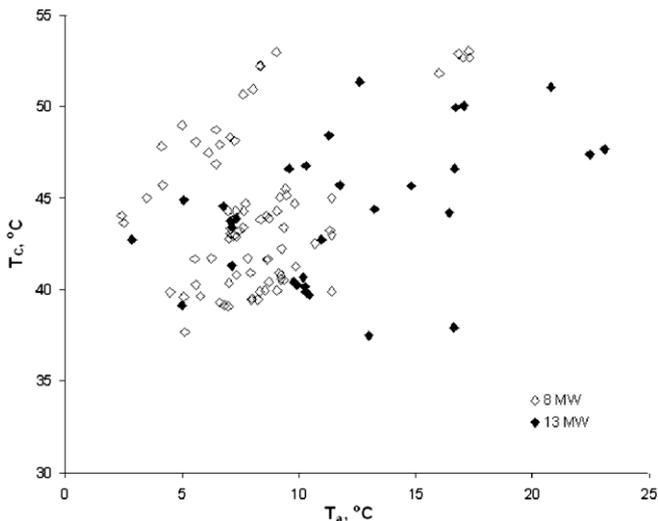
Fig. 5. Steam condensing temperature in dry condenser versus ambient temperature for two steam turbine outputs.
