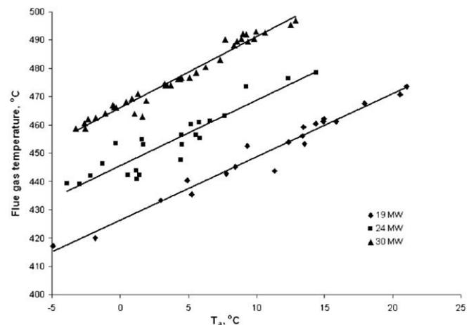
Fig. 7. Temperature of flue gases exiting gas turbine as a function of ambient temperature for three typical gas turbine power outputs.
