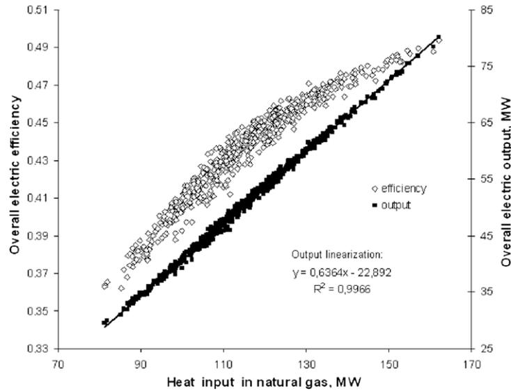
Fig. 4. Overall electric efficiency and overall electric output plotted as functions of heat input in natural gas.
