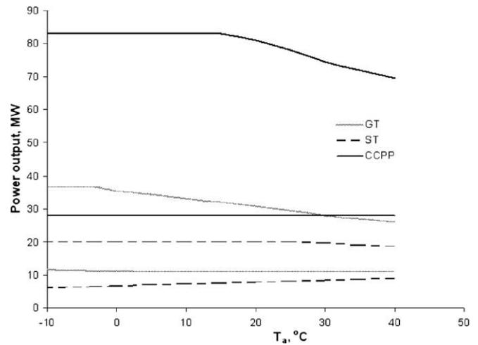
Fig. 2. Operation limits of gas turbines and steam turbine; typical lower and upper load limit of combined cycle.
