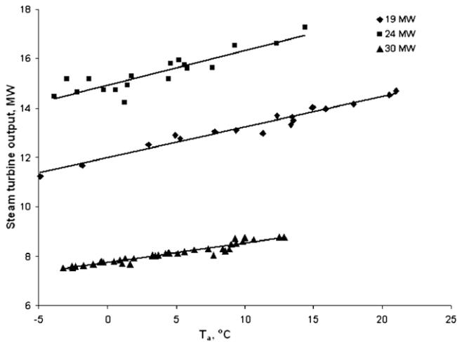
Fig. 9. Steam turbine output as a function of ambient temperature for three typical gas turbine outputs. Squares and diamonds: both gas turbines are in operation. Triangles: only one gas turbine operates.
