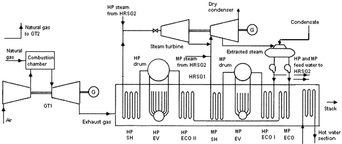
Fig. 1. Scheme of combined cycle power plant studied.
