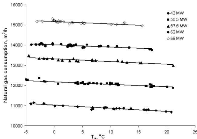
Fig. 10. Natural gas consumption needed to achieve specific combined cycle's outputs (see legend) as a function of ambient temperature.
