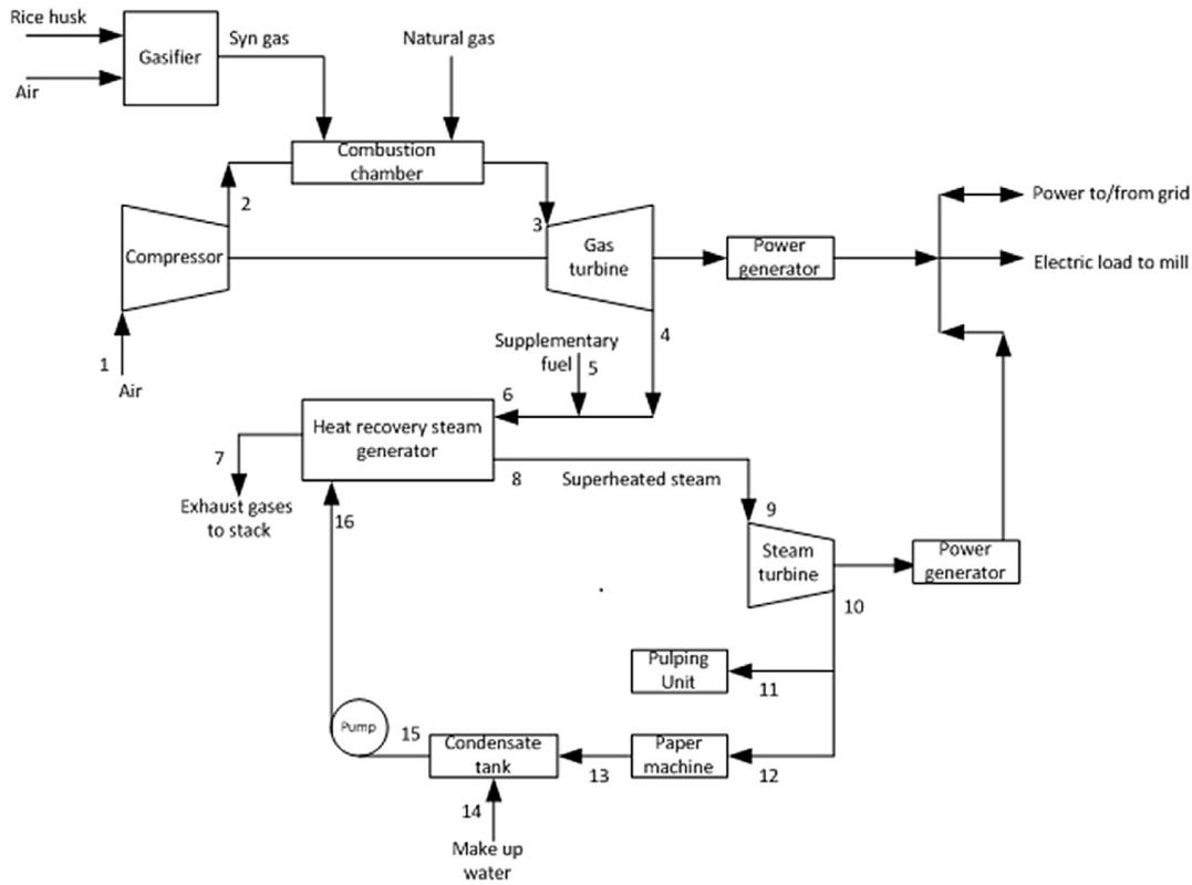
Fig. 6 – Schematic diagram of the proposed combined cycle cogeneration system.
