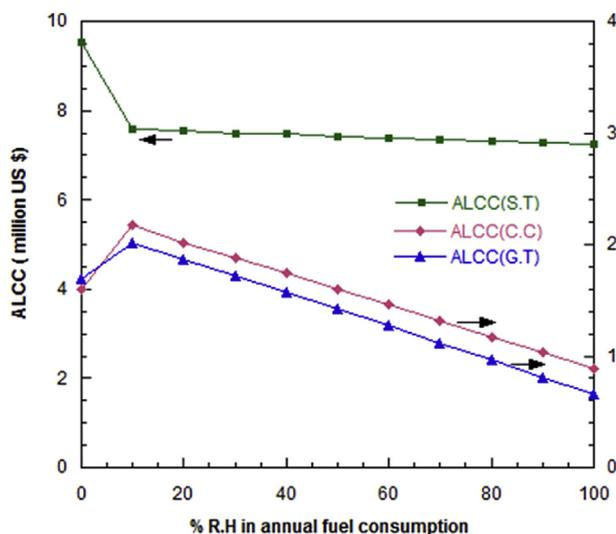
**Fig. 7 – Variation of the annualised life cycle cost (ALCC) with the fuel ratio in terms of the percentage of rice husk (% R.H) for different CHP options.**
