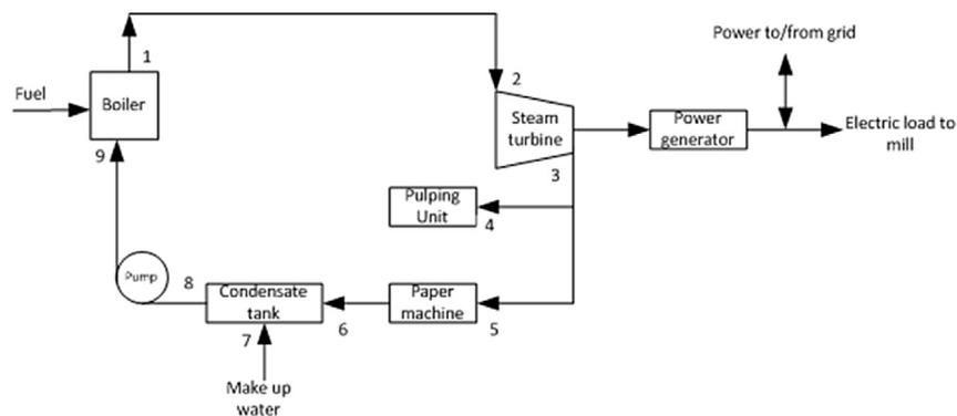
Fig. 3 – Schematic diagram of the proposed steam turbine cogeneration system.
