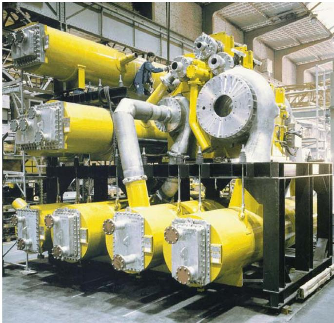
Figure 5 – Integrally Geared Compressor
