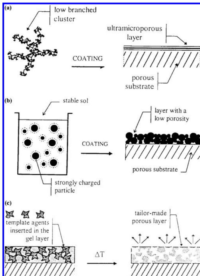
**Figure 3.** Schematic of the three important sol–gel routes used for preparation of microporous membranes.<sup>246,299</sup> (Reprinted with permission from ref 246. Copyright 2002 Taylor & Francis Group, LLC, <http://www.taylorandfrancis.com>.)
