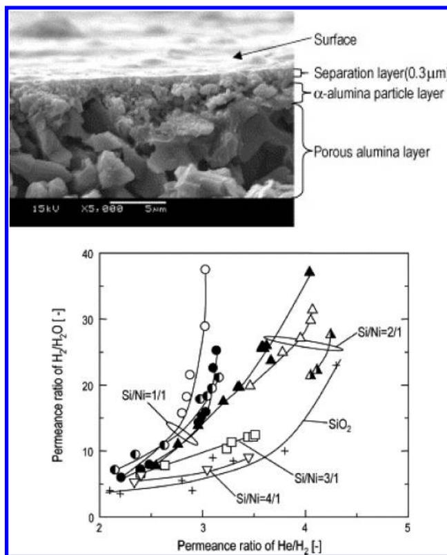
**Figure 5.** (a) Cross section of a Ni-doped silica membrane (Si/Ni = 2/1). (b) Observed permeance ratio of H<sub>2</sub>/H<sub>2</sub>O vs the permeance ratio of He/H<sub>2</sub> for nine membranes (Si/Ni = 0–1/1) at 500 °C. (Reprinted from ref 244, copyright 2006, Elsevier.)
