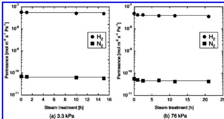
**Figure 4.** Steam stability for a silica membrane prepared at 600 °C.<sup>199</sup> (Reprinted from ref 199, copyright 2005, with permission from Elsevier.)
