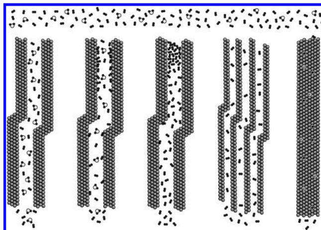
**Figure 1.** Illustration of five H<sub>2</sub> separation mechanisms: (i) Knudson diffusion; (ii) surface diffusion; (iii) capillary condensation; (iv) molecular sieving; (v) solution diffusion.
