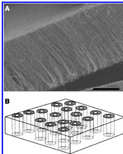
**Figure 8.** (A) An as-grown, dense, multiwalled CNT array. Scale bar, 50  $\mu\text{m}$ . (B) Schematic of the target membrane structure. With a polymer embedded between the CNTs, a viable membrane structure can be readily produced, with the pore being the rigid inner-tube diameter of the CNT.<sup>370</sup> (From ref 370 (<http://www.sciencemag.org>). Reprinted with permission from AAAS.)
