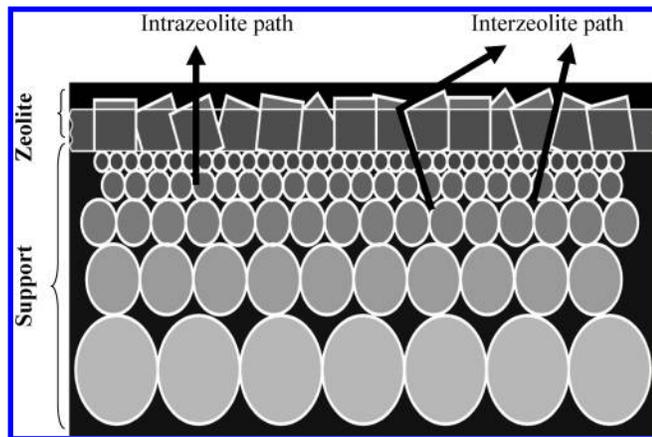
**Figure 6.** Not-to-scale representation of a zeolite membrane on a nonselective oxide support (i.e.,  $\text{Al}_2\text{O}_3$ ), showing possible permeation pathways, either interzeolite crystals or intrazeolite crystals.
