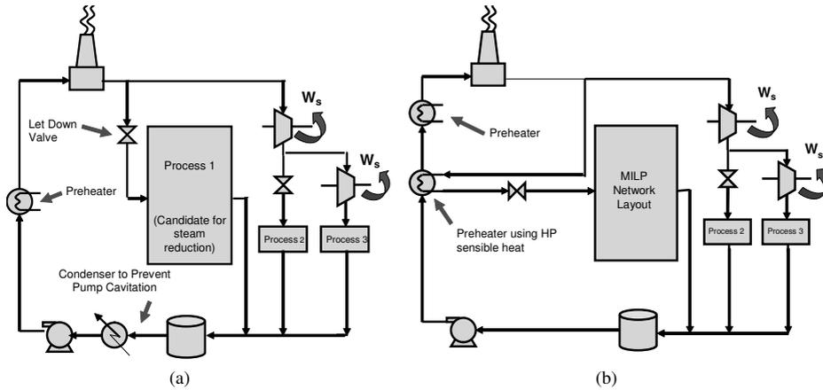
Figure 1: Steam system layouts.
