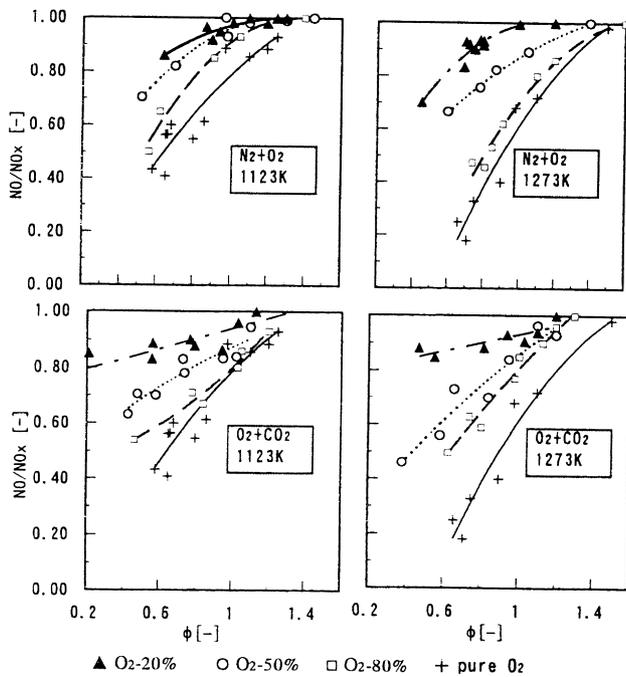
Fig. 4. The effect of fuel equivalence ratio and O<sub>2</sub> concentration on NO/NO<sub>x</sub> for N<sub>2</sub>- and CO<sub>2</sub>-based inlet gases at 1123 and 1273 K.
