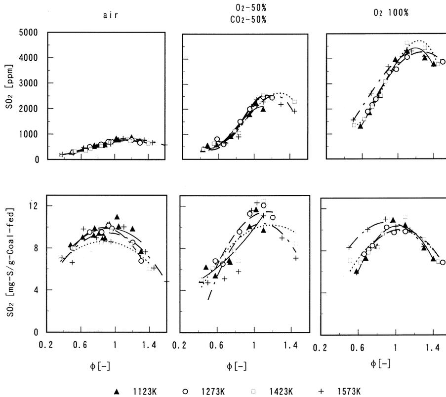
Fig. 9. SO<sub>2</sub> emissions versus equivalence ratio and temperature at different O<sub>2</sub> concentration for N<sub>2</sub>- and CO<sub>2</sub>-based inlet gases.
