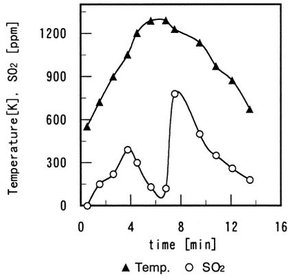
Fig. 6. Changes of temperature and SO<sub>2</sub> emission in batch combustion.
