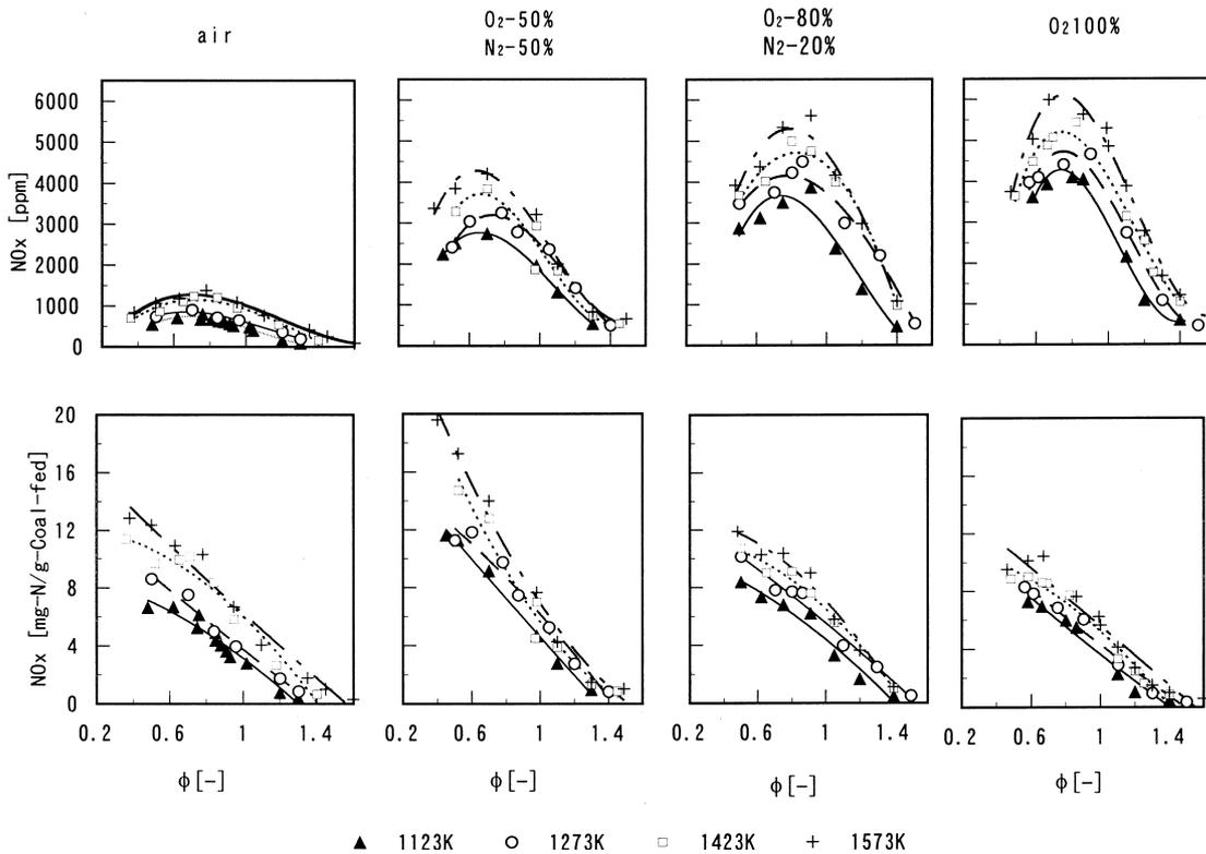
Fig. 7. NO<sub>x</sub> emissions versus equivalence ratio and temperature at different O<sub>2</sub> concentration for N<sub>2</sub>-based inlet gases.
