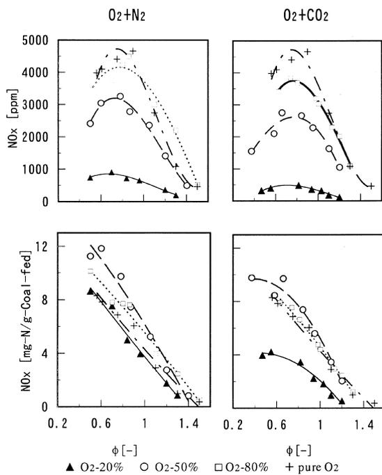
Fig. 3. NO<sub>x</sub> emission versus fuel equivalence ratio at different O<sub>2</sub> concentrations for N<sub>2</sub>- and CO<sub>2</sub>-base inlet gases at 1273 K.
