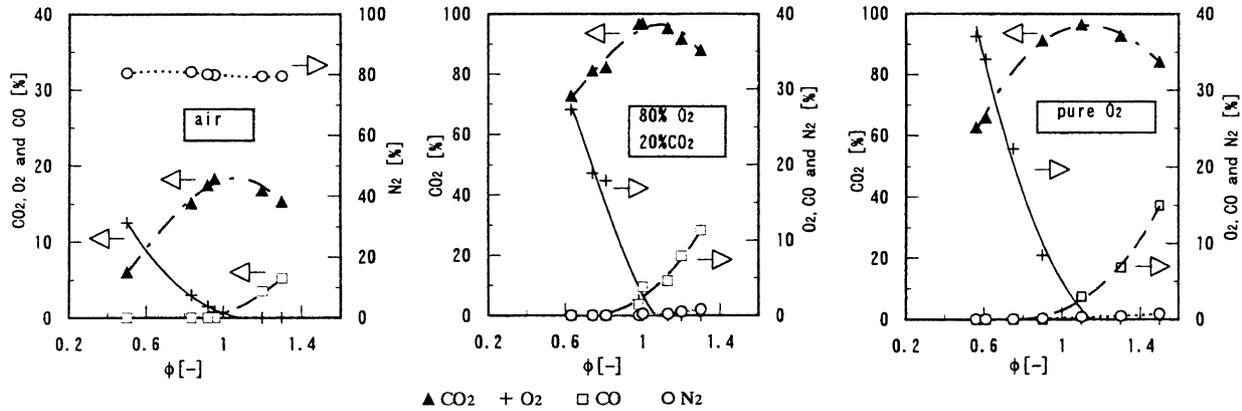
Fig. 2. The variations of O<sub>2</sub>, CO<sub>2</sub>, N<sub>2</sub> and CO in flue gas with fuel equivalence ratio at 1273 K.
