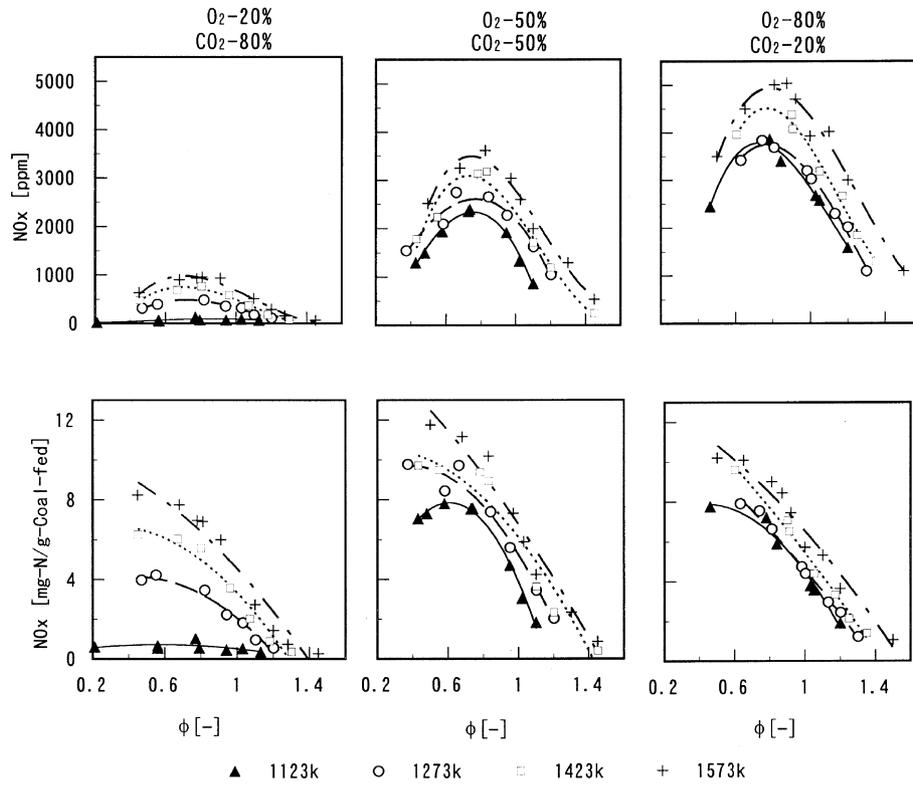
Fig. 8. NO<sub>x</sub> emissions versus equivalence ratio and temperature at different O<sub>2</sub> concentration for CO<sub>2</sub>-based inlet gases.
