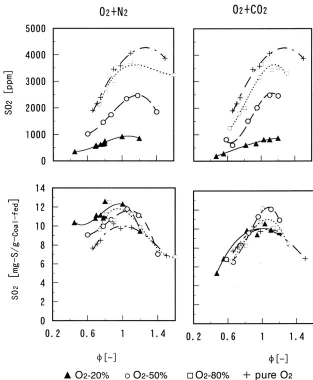
Fig. 5. SO<sub>2</sub> emission versus fuel equivalence ratio at different O<sub>2</sub> concentrations for N<sub>2</sub>- and CO<sub>2</sub>-based inlet gases at 1273 K.
