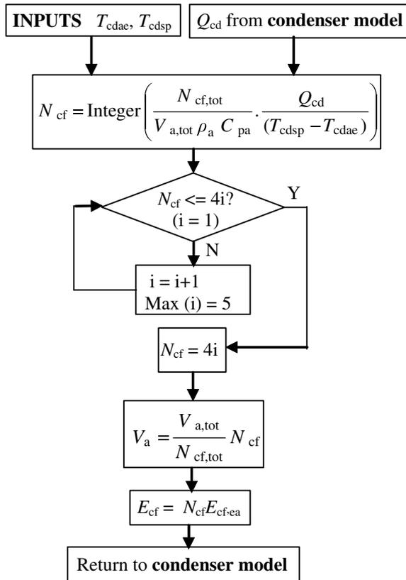
Fig. 1. Procedure for determining the number and power of the staged condenser fans with constant speed.
