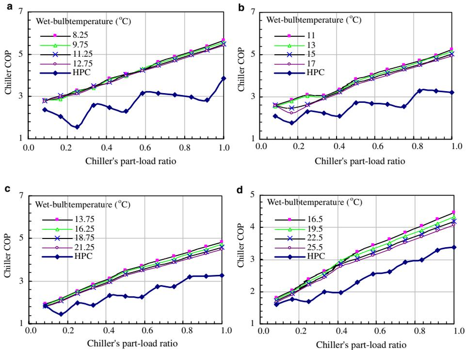
Fig. 6. Improved chiller's COP in various operating conditions at different combinations of dry-bulb and wet-bulb temperatures of outdoor air: (a) outdoor temperature = 15 °C; (b) outdoor temperature = 20 °C; (c) outdoor temperature = 25 °C; (d) outdoor temperature = 30 °C.
