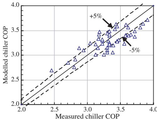
Fig. 4. Comparison between the modelled and measured data of the chiller coefficient of performance (COP).
