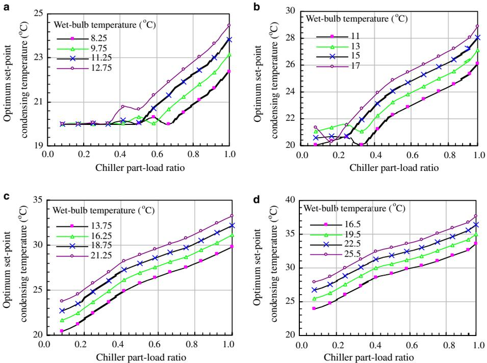
Fig. 5. Optimum set points of condensing temperature at different combinations of dry-bulb and wet-bulb temperatures of outdoor air: (a) outdoor temperature = 15 °C; (b) outdoor temperature = 20 °C; (c) outdoor temperature = 25 °C; (d) outdoor temperature = 30 °C.
