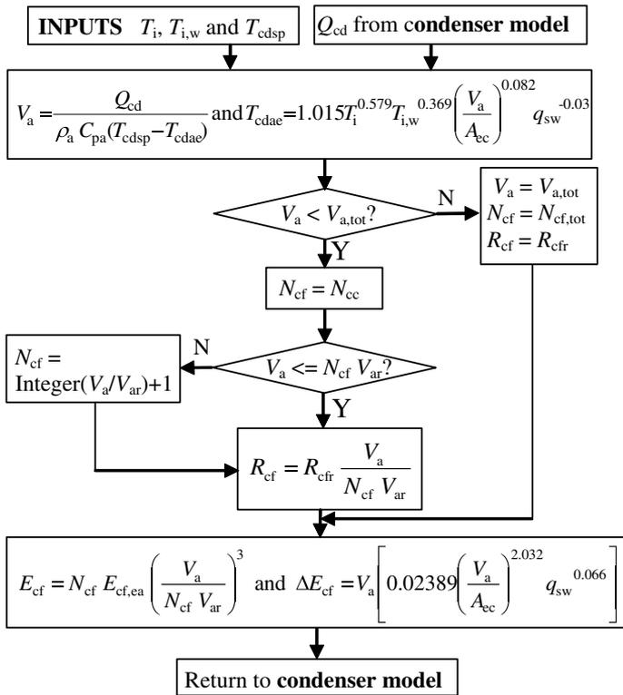
Fig. 2. Procedure for evaluating the number, speed and power of staged condenser-fans.
