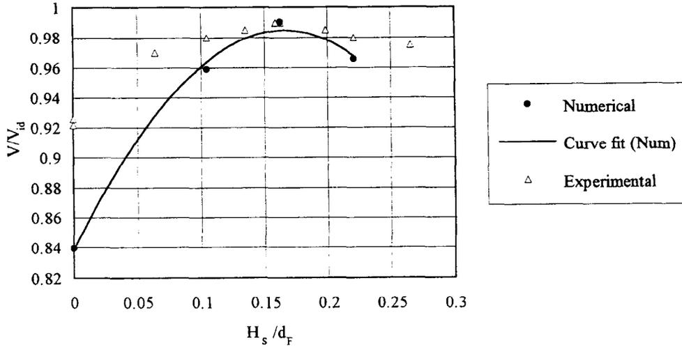
Fig. 8. The effect of the length of the cylindrical inlet shroud on the fan performance.
