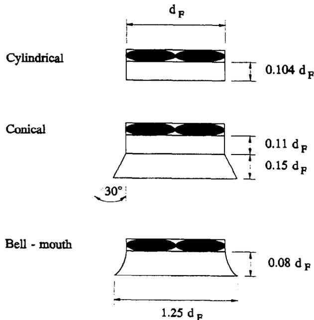
Fig. 5. The dimensions of the three fan inlet shrouds.
