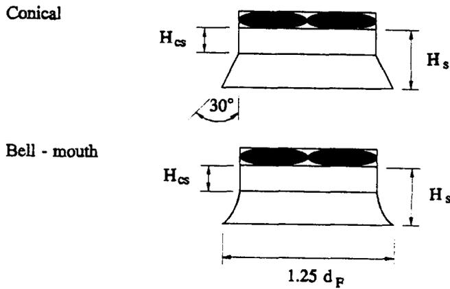
Fig. 10. Diagram of a conical inlet shroud and a bell-mouth inlet shroud.
