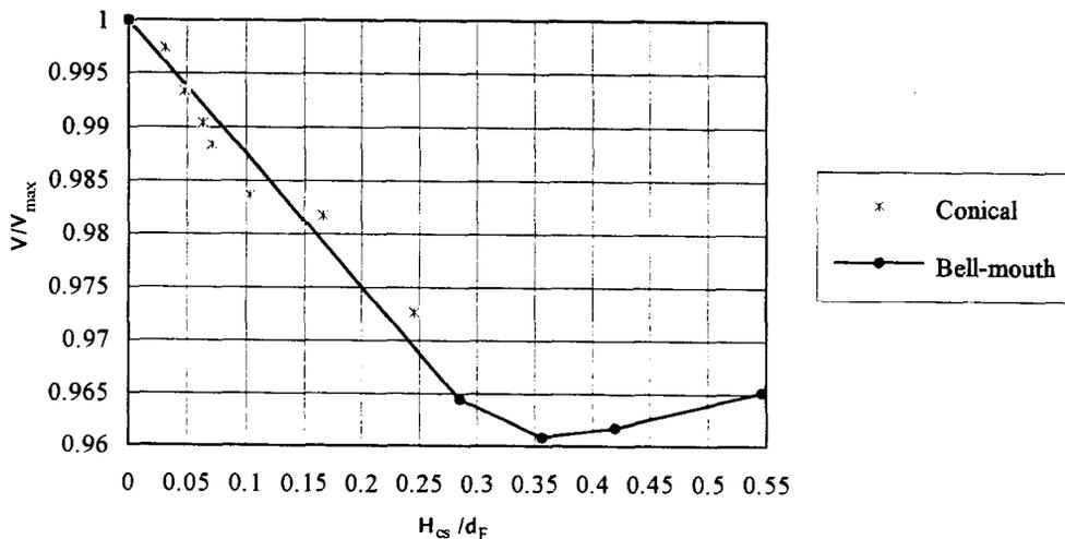
Fig. 11. The effect of a cylindrical section as part of a conical and bell-mouth inlet shroud on fan performance.
