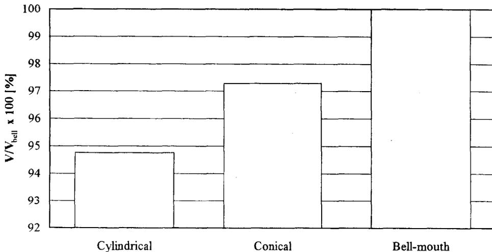
Fig. 7. A comparison between the volume flow rates for the three different fan systems.
