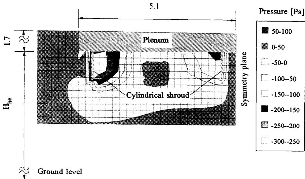
Fig. 9. A pressure contour plot at the inlet to the cylindrical fan inlet shroud.
