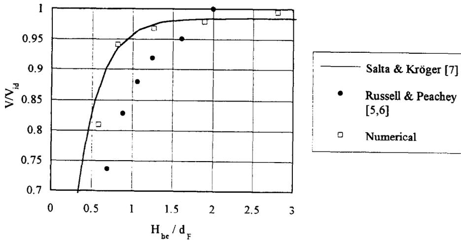
Fig. 4. The effect of the ACHE platform height on the fan performance.
