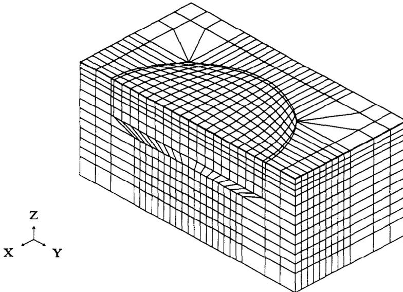
Fig. 3. A section of the computational grid around the fan.
