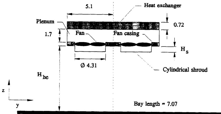
Fig. 2. A single bay of a long ACHE bank (dimensions in metres).
