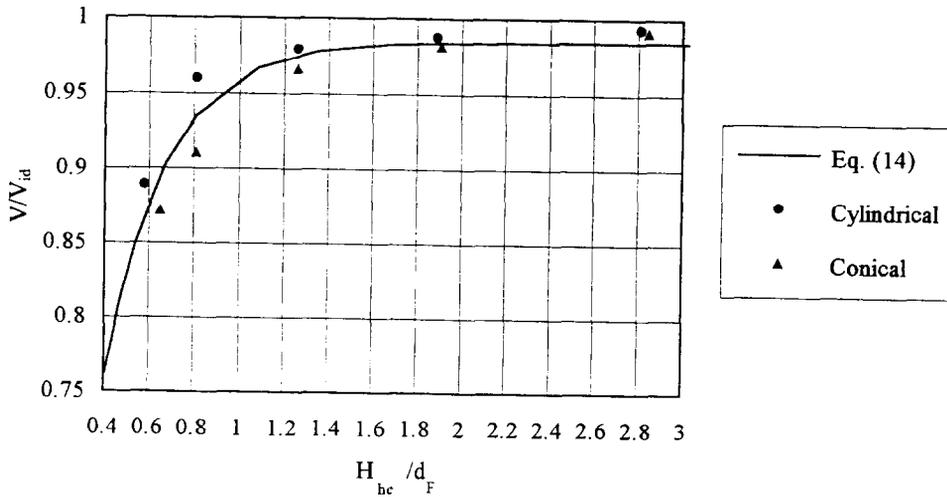
Fig. 6. The effect of ACHE platform height on the fan performance.
