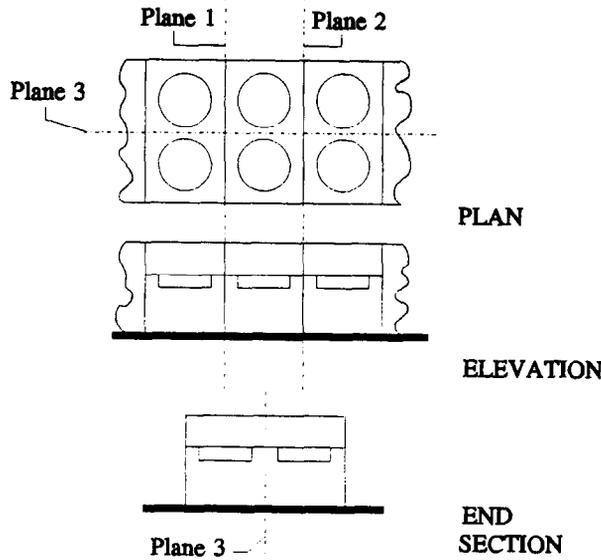
Fig. 1. Diagram of a long ACHE bank showing the planes over which flow will not occur.
