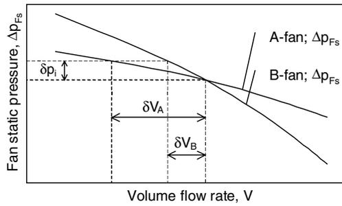
Fig. 9. Effect of inlet flow distortion on the volume flow rate of the A-fan and B-fan.
