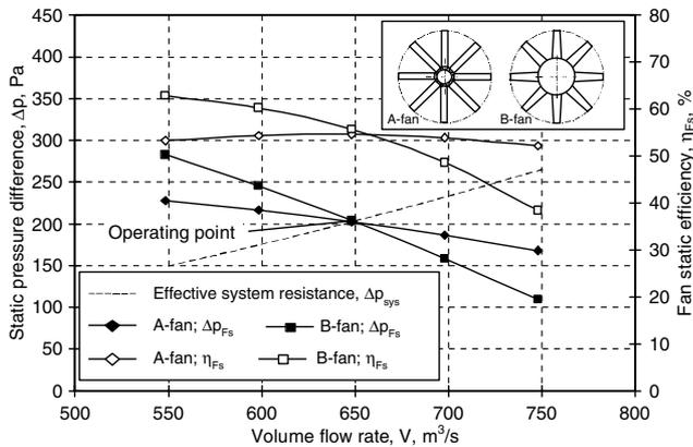
Fig. 6. Numerically determined fan characteristics and ideal operating point.
