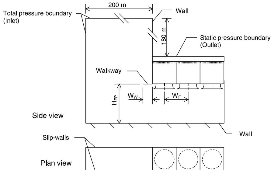
Fig. 5. Computational geometry and boundary conditions.
