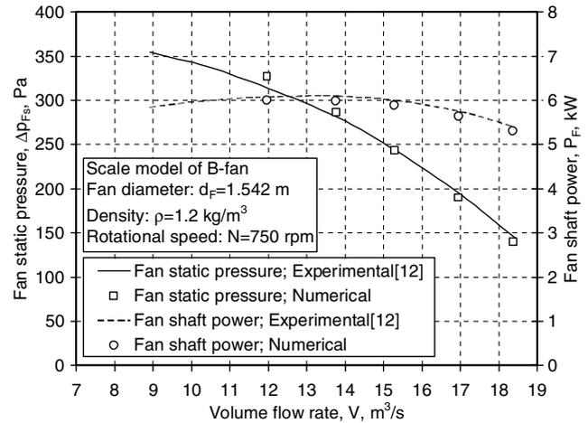
Fig. 4. Numerical prediction of the fan characteristics for a scale model B-fan.
