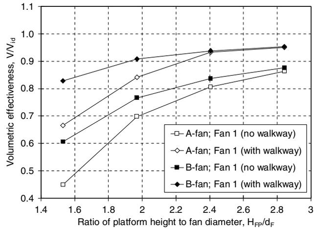
Fig. 10. Effect of a walkway on volumetric effectiveness of the edge fan.
