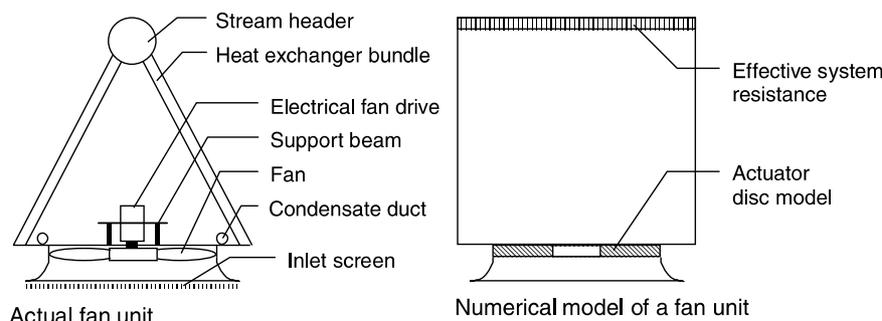
Fig. 2. Numerical model of a typical fan unit in the ACSC.
