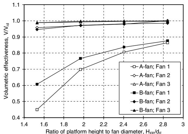
Fig. 8. Volumetric effectiveness of fans 1–3 for the A-fan and B-fan.
