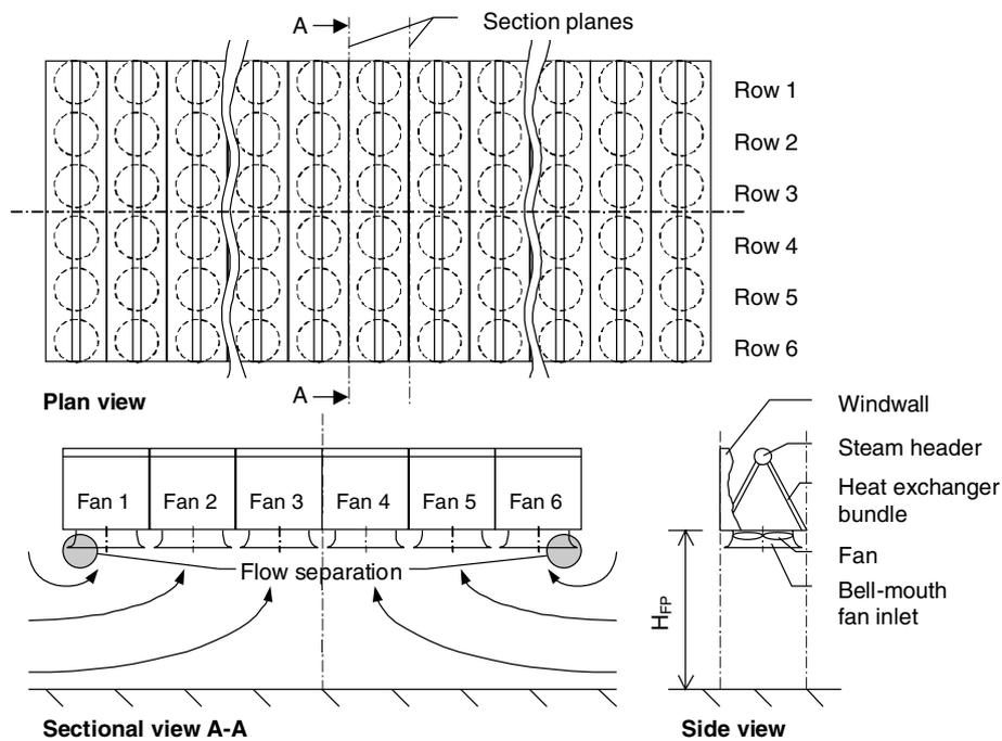
Fig. 1. Schematic of a representative section of a long ACSC depicting the induced cross-draft and resulting flow separation at the inlets of the periphery fans.
