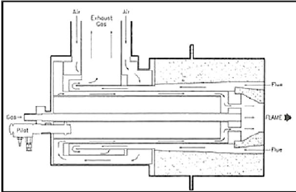
Fig. 2 Principle of recuperative burner system [4]
