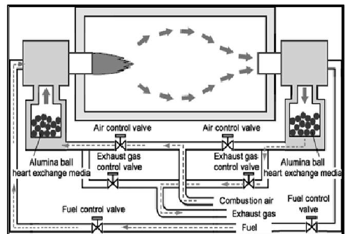
Fig. 1 Principle of regenerative burner system [2]
