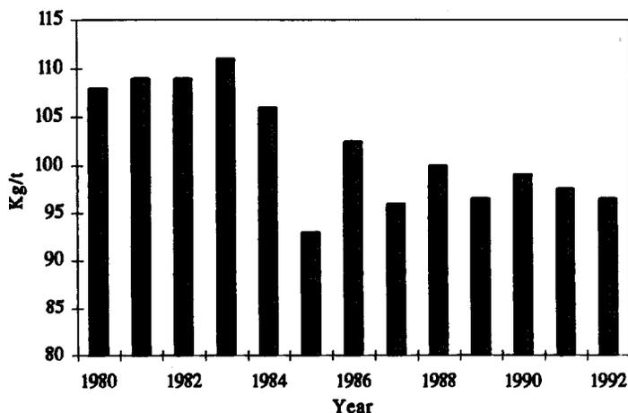
Fig. 1. Annual fuel oil consumption of the flash calciner.
