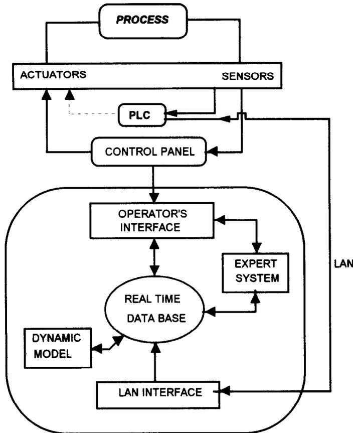
Fig. 7. Structure of the control system.
