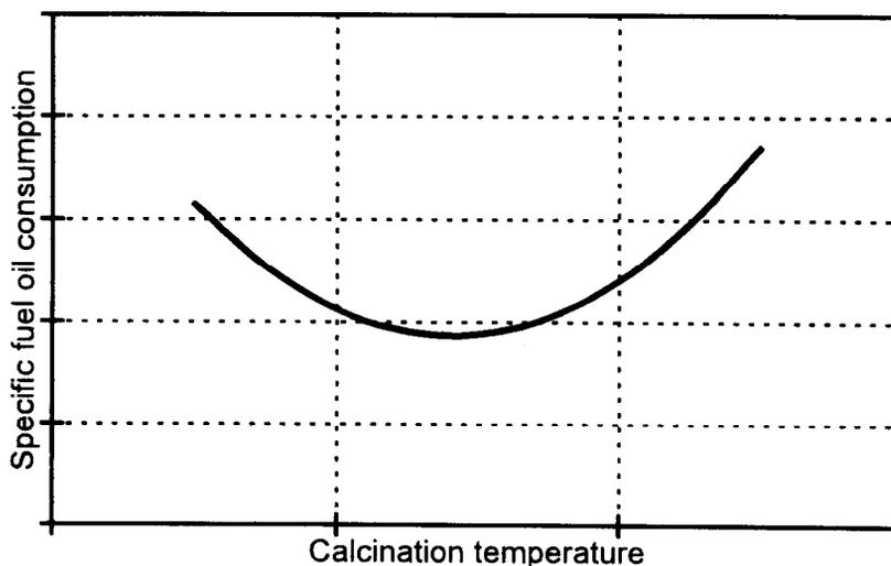
Fig. 4. Specific fuel consumption vs calcination temperature.
