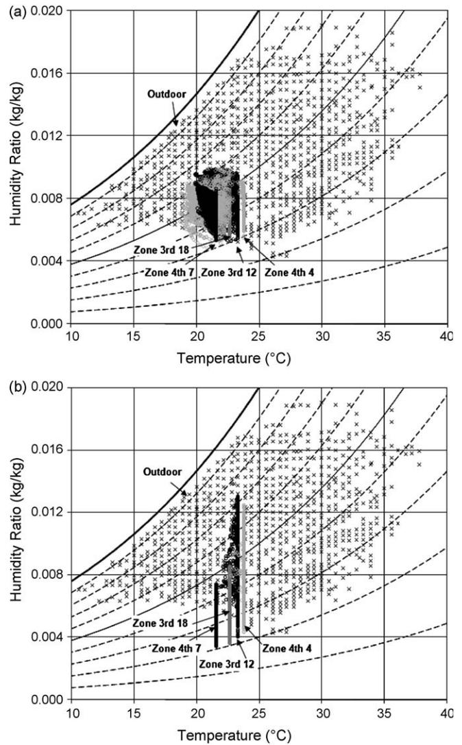
Fig. 5. Comparison of the indoor conditions for Case II, (a) VAV system, (b) VRF system.
