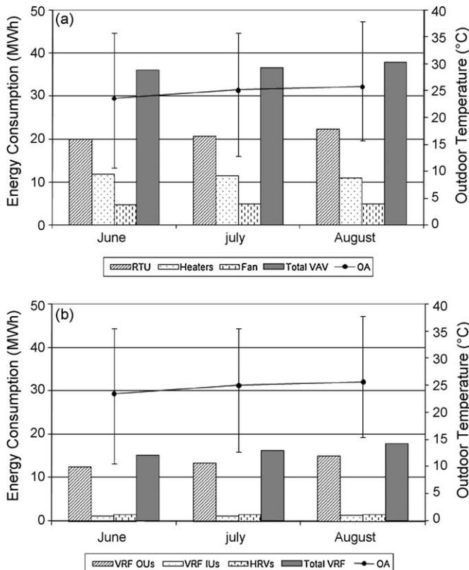
**Fig. 6.** Monthly energy consumption of the VAV and VRF systems for Case III, (a) VAV system, (b) VRF system.
