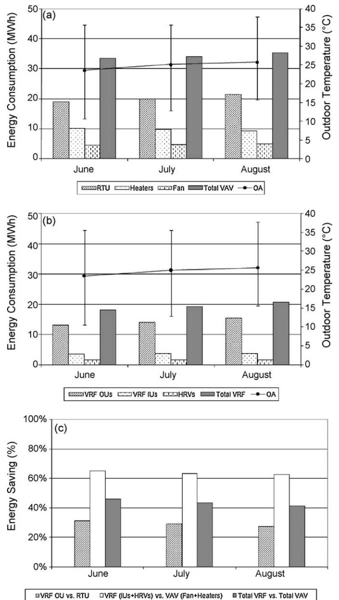
**Fig. 2.** Monthly energy consumption of the VAV and VRF systems and the energy-saving potential of the VRF system, (a) VAV system, (b) VRF system, (c) energy-saving potential of the VRF system.
