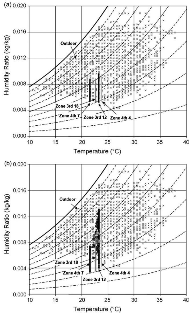
**Fig. 7.** Comparison of the indoor conditions for Case III, (a) VAV system, (b) VRF system.
