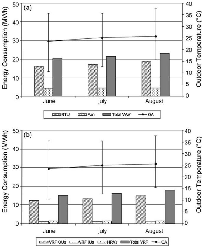
Fig. 4. Monthly energy consumption of the VAV and VRF systems for Case II, (a) VAV system, (b) VRF system.
