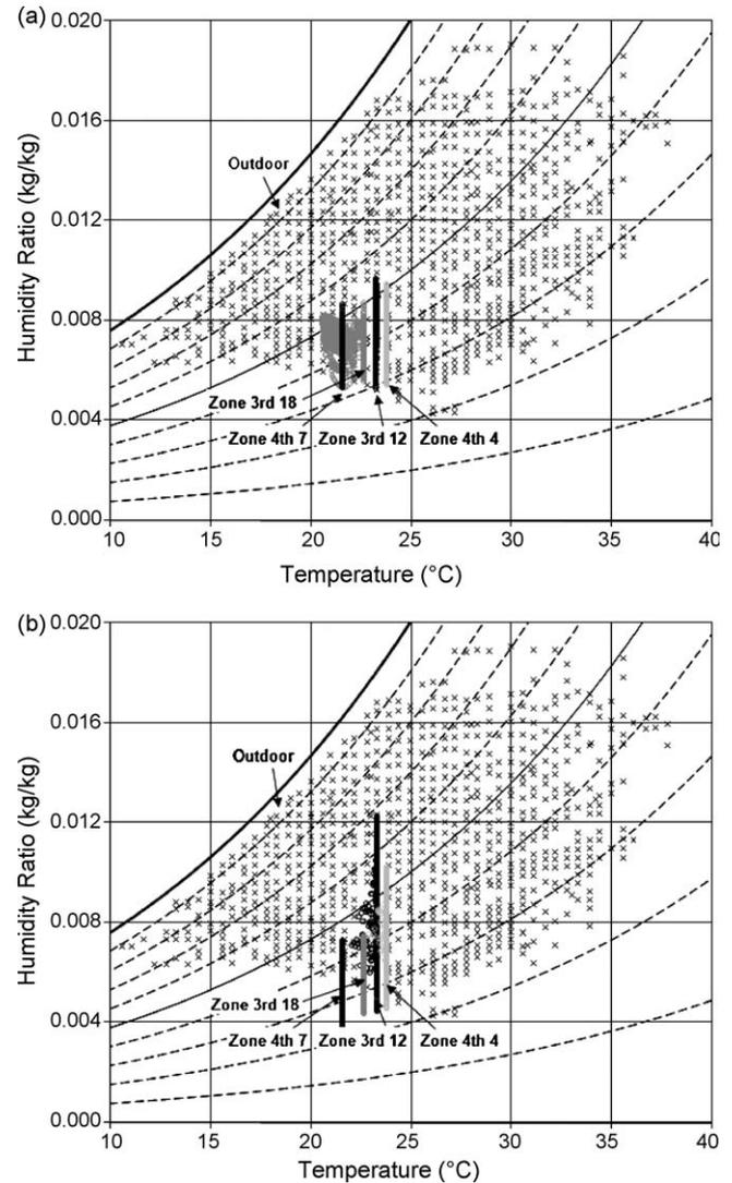
Fig. 3. Comparison of the indoor conditions for Case I. (a) VAV system, (b) VRF system.
