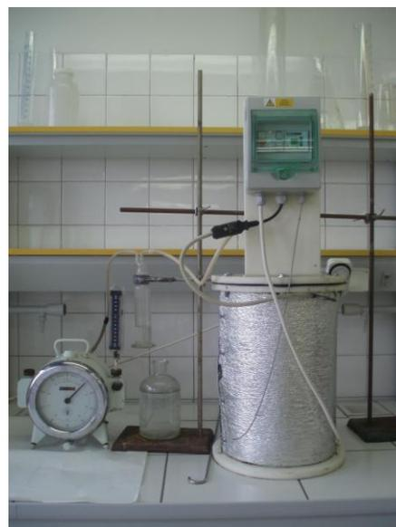
**Figure 1** Laboratory model of anaerobic reactor
