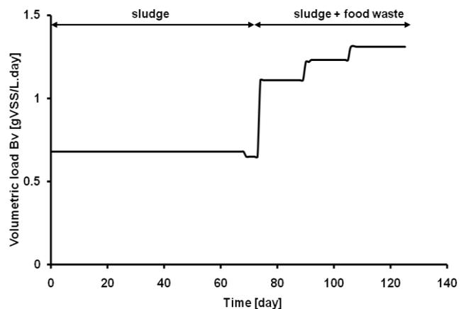
**Figure 3** Development of organic load during the co-digestion laboratory test.
