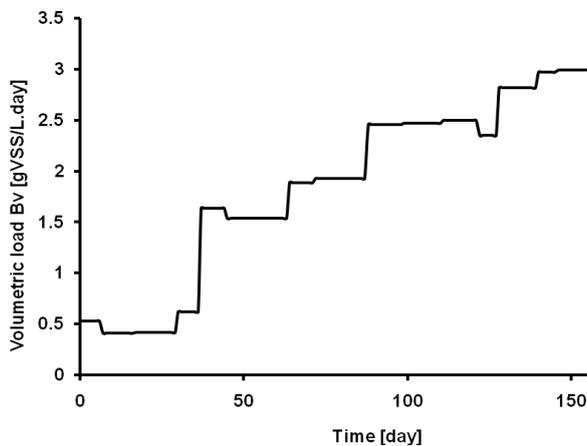
**Figure 2** Development of organic load during the methanogenic laboratory test.
